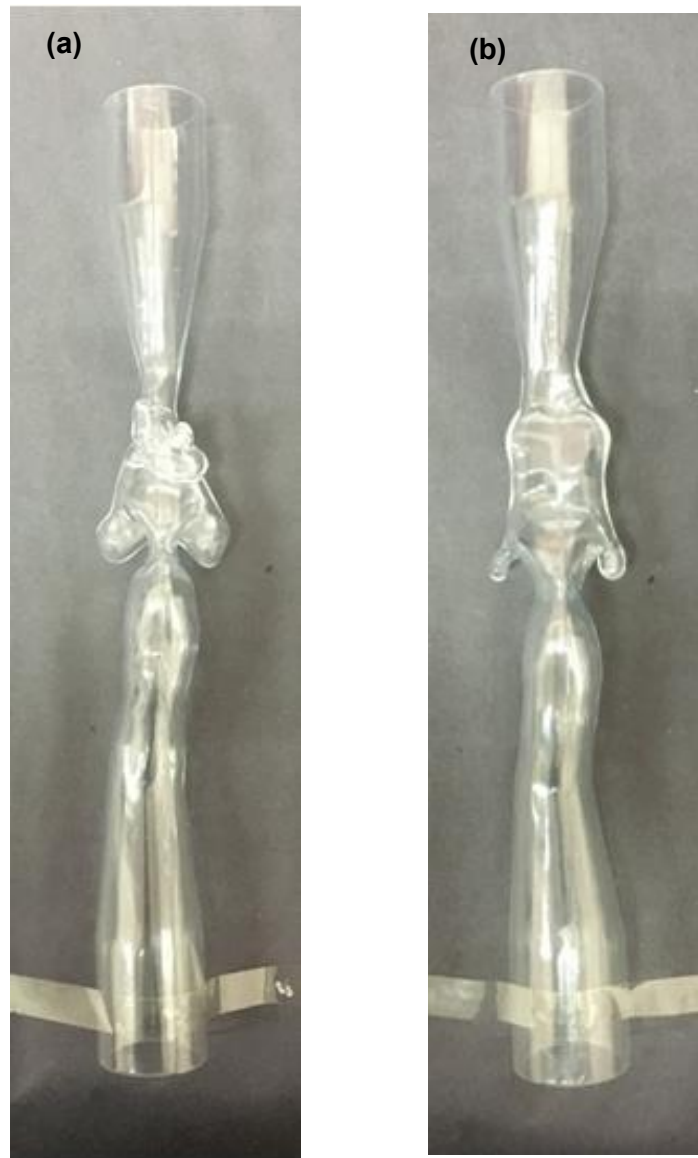
Figure 8.6: The transparent pharynx model produced from the Stereolithography machine: (a) pre-operative model and (b) post-operative model.
