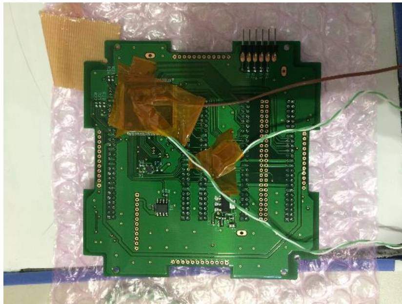
Figure 5-7. Thermocouples placed on the CPLD of SoftCIB
