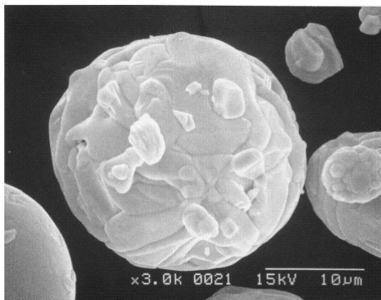
Fig. 2. Surface morphology of (\text{Bi}_2\text{Te}_3)_{0.2}(\text{Sb}_2\text{Te}_3)_{0.8} compounds powders by SEM.
