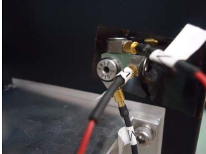
Figure 2.3.3: The view of attachment of the accelerometers.
