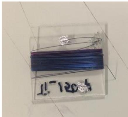
Figure 10. Ti wire sample used for XRD analysis
