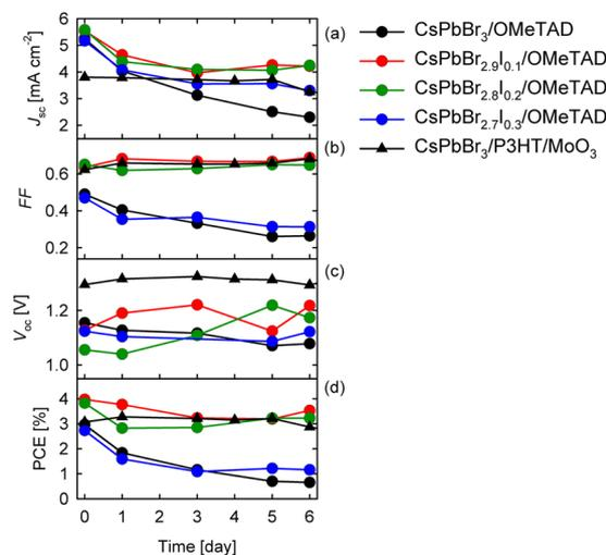
**Figure 7.** Aging analysis of CsPbBr<sub>3-x</sub>I<sub>x</sub> devices ( $x$  varies between 0, 0.1, 0.2, and 0.3 molar ratio). Figures show the cell parameters (a)  $J_{sc}$ , (b)  $FF$ , (c)  $V_{oc}$ , and (d) efficiency as a function of time.
