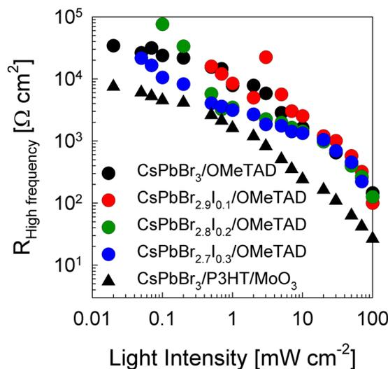
**Figure 6.** Resistance fitted at high frequency range in impedance spectroscopy measured at numerous light intensities from low light intensity to 1 sun illumination. Different CsPbBr<sub>3-x</sub>I<sub>x</sub> perovskite compositions ( $x$  varies between 0, 0.1, 0.2, and 0.3 in molar ratio) and hole transport materials as *spiro*-OMeTAD/Au (circle dots) and P3HT/MoO<sub>3</sub>/Au (triangle dots) were analyzed.
