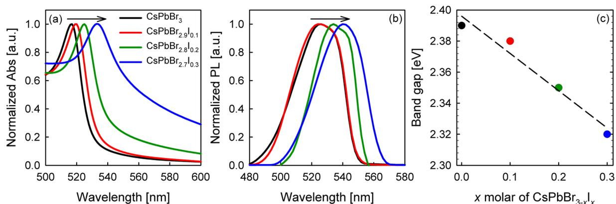
**Figure 1.** Normalized (a) absorption (Abs) and (b) photoluminescence (PL) of CsPbBr<sub>3-x</sub>I<sub>x</sub>, where  $x$  is 0, 0.1, 0.2, and 0.3 in molar ratio. The intersection between Abs and PL spectra represents the (c) band gap energy.
