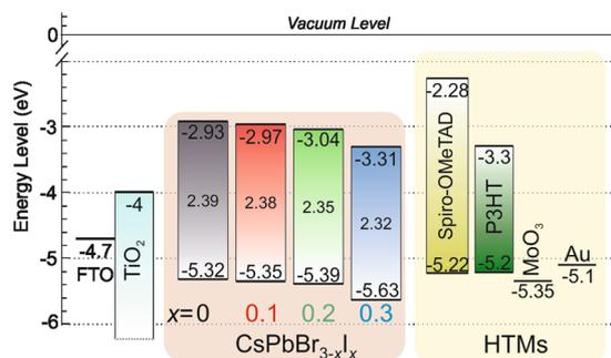
**Figure 2.** Schematic energy level diagram of a complete  $\text{TiO}_2$ -mesoporous  $\text{CsPbBr}_{3-x}\text{I}_x$  ( $x$  is 0, 0.1, 0.2 or 0.3) perovskite solar cell, employing either *spiro*-OMeTAD<sup>34</sup> or P3HT/MoO<sub>3</sub><sup>32,35</sup> as the hole transporting material. The band gap of each perovskite, where  $x$  is 0, 0.1, 0.2, and 0.3 was also indicated.
