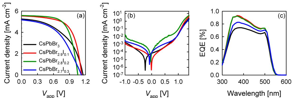
**Figure 3.** (a) J-V measurements under simulated AM1.5G sun light of 100 mW cm<sup>-2</sup> irradiance, and (b) under dark. (c) Represents the EQE for glass/FTO/c-TiO<sub>2</sub>/mp-TiO<sub>2</sub>/CsPbBr<sub>3-x</sub>I<sub>x</sub>/spiro-OMeTAD/Au solar cells, where  $x$  varies in 0, 0.1, 0.2, and 0.3 molar ratio.
