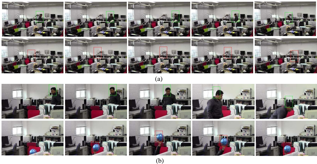
Fig. 10. Performance of head detection and tracking. The green box shows that the proposed system detects a motion and a head, the red box shows that the system detects a motion but not a head. (a) Scene 1: The system can distinguish a head and a racket. (b) scene 2: The system can distinguish a head and a ball
