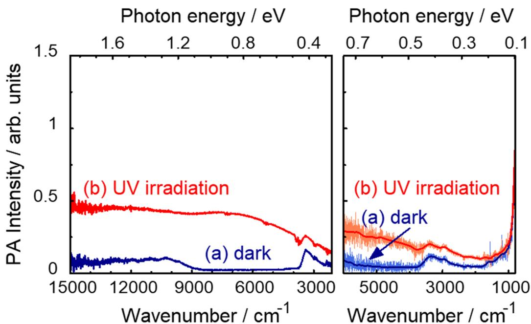
**Figure 5.** FTIR-PAS spectra of rutile  $\text{TiO}_2$  powder (MT-600B) under  $\text{N}_2+\text{EtOH}$  (a) before and (b) during UV irradiation. Measurements were carried out by using FT-NIR (left) and FT-MIR (right) spectrometers.
