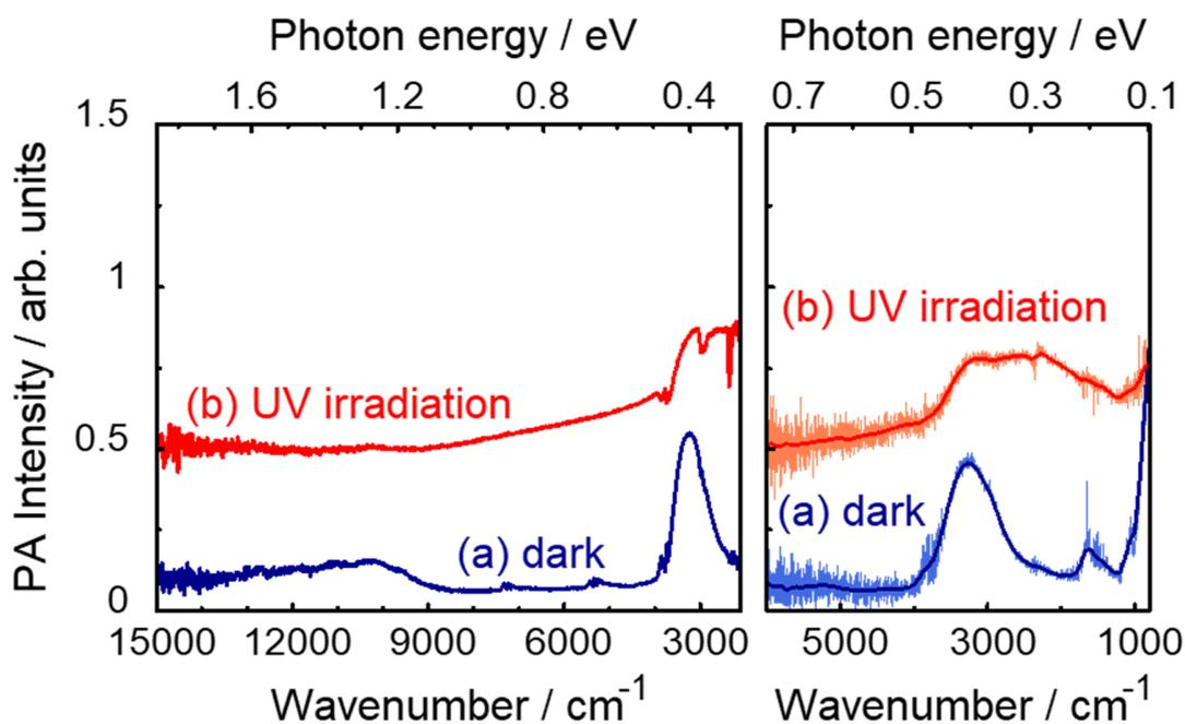
**Figure 1.** FTIR-PAS spectra of anatase  $\text{TiO}_2$  powder (AMT-100) under  $\text{N}_2+\text{EtOH}$  (a) before and (b) during UV irradiation. Measurements were carried out by using FT-NIR (left) and FT-MIR (right) spectrometers.
