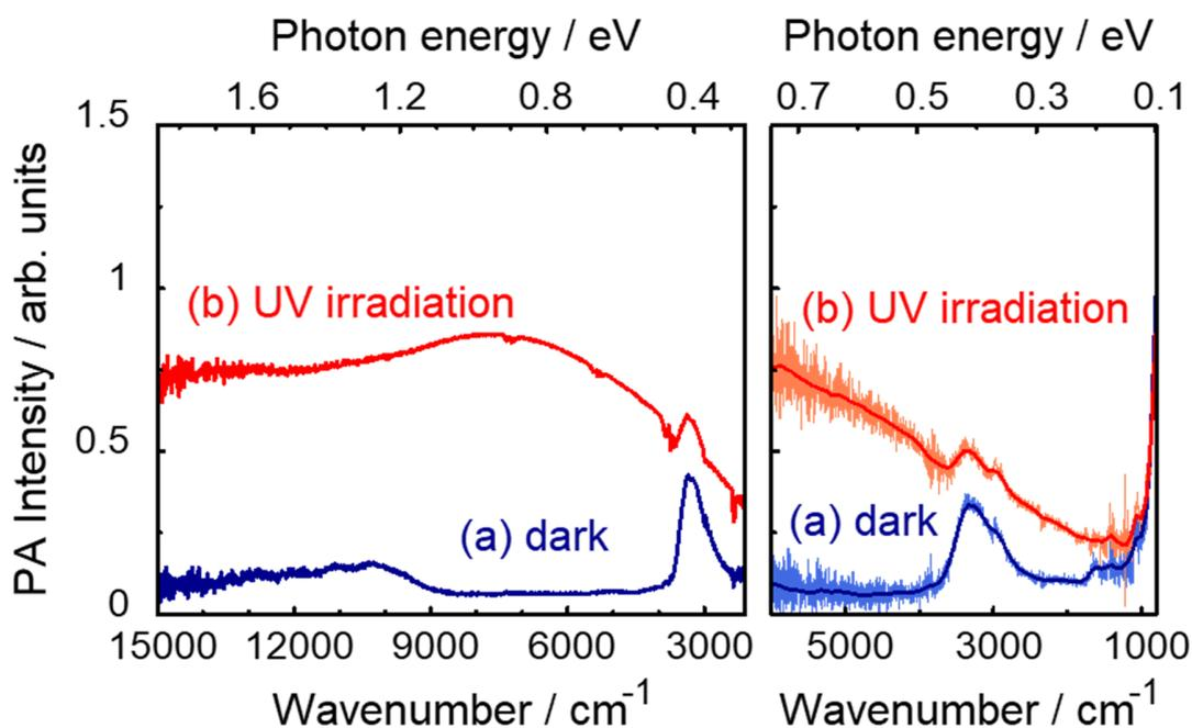
**Figure 4.** FTIR-PAS spectra of rutile TiO<sub>2</sub> powder (MT-150A) under N<sub>2</sub>+EtOH (a) before and (b) during UV irradiation. Measurements were carried out by using FT-NIR (left) and FT-MIR (right) spectrometers.
