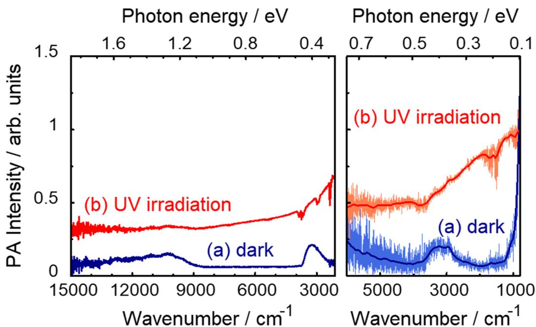
**Figure 3.** FTIR-PAS spectra of anatase TiO<sub>2</sub> powder (AMT-600) under N<sub>2</sub>+EtOH (a) before and (b) during UV irradiation. Measurements were carried out by using FT-NIR (left) and FT-MIR (right) spectrometers.
