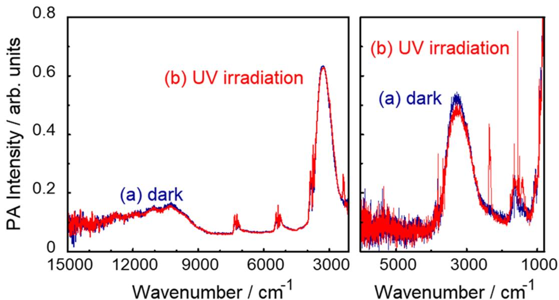
**Figure 2.** FTIR-PAS spectra of anatase TiO<sub>2</sub> powder (AMT-100) under O<sub>2</sub>+EtOH (a) before and (b) during UV irradiation. Measurements were carried out by using FT-NIR (left) and FT-MIR (right) spectrometers.
