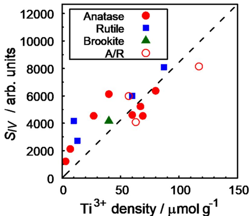
**Figure 7.** Relation between  $S_{IV}$  and  $Ti^{3+}$  density. Filled circles, filled squares, filled triangle and open circles denote anatase, rutile, brookite and a mixture of anatase and rutile (A/R, predominantly anatase), respectively.
