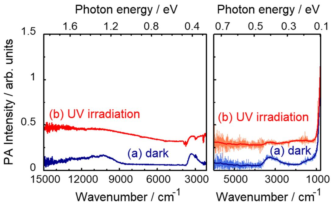
**Figure 6.** FTIR-PAS spectra of brookite  $\text{TiO}_2$  powder under  $\text{N}_2+\text{EtOH}$  (a) before and (b) during UV irradiation. Measurements were carried out by using FT-NIR (left) and FT-MIR (right) spectrometers.
