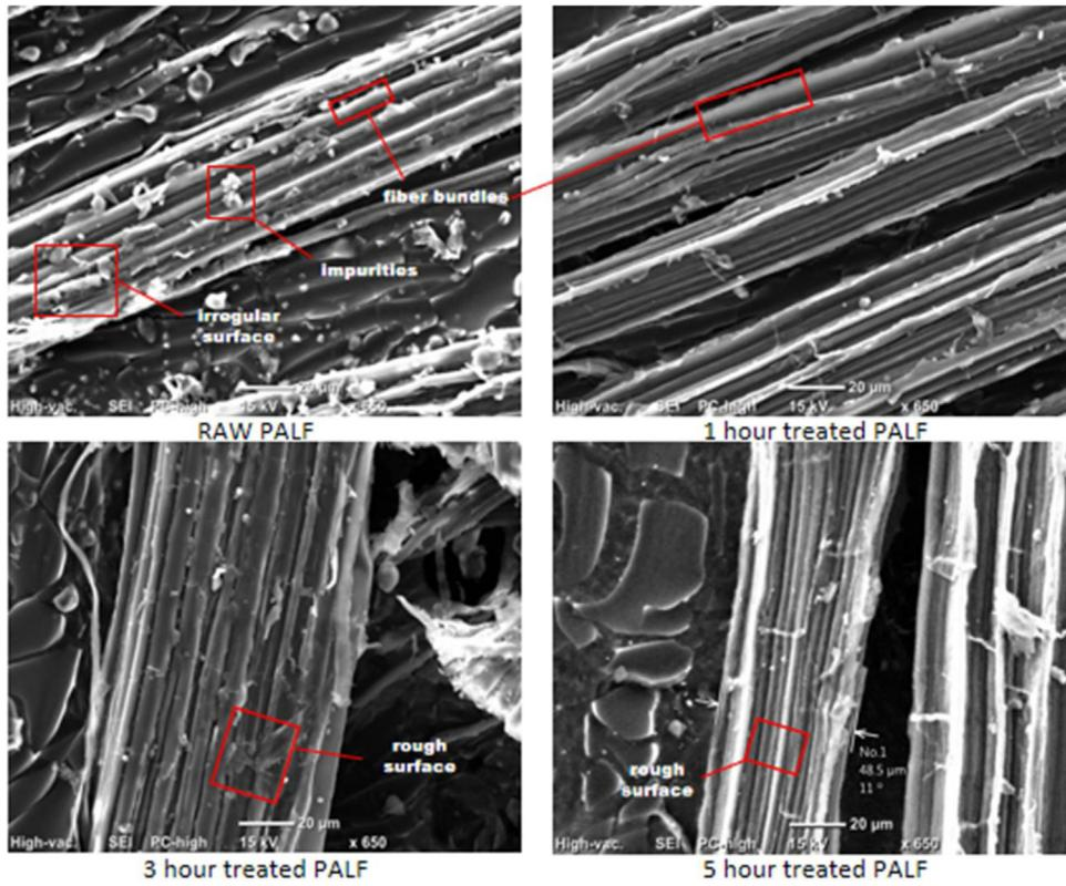
Fig. 2 – SEM image of untreated and treated fiber.
