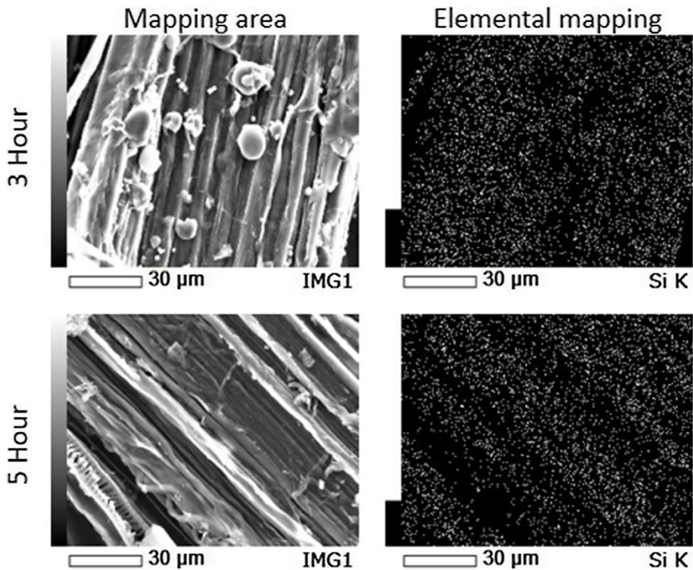
Fig. 3 – Si element mapping through EDX.
