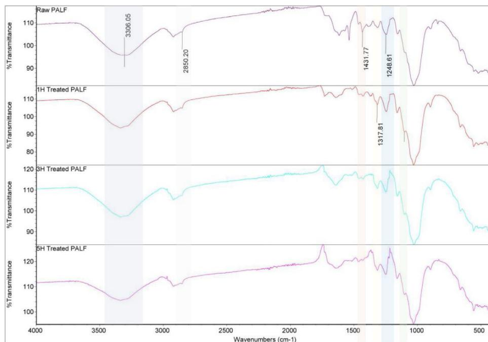
**Fig. 7 – The results of FTIR(ATR) on treated and untreated PALF.**
