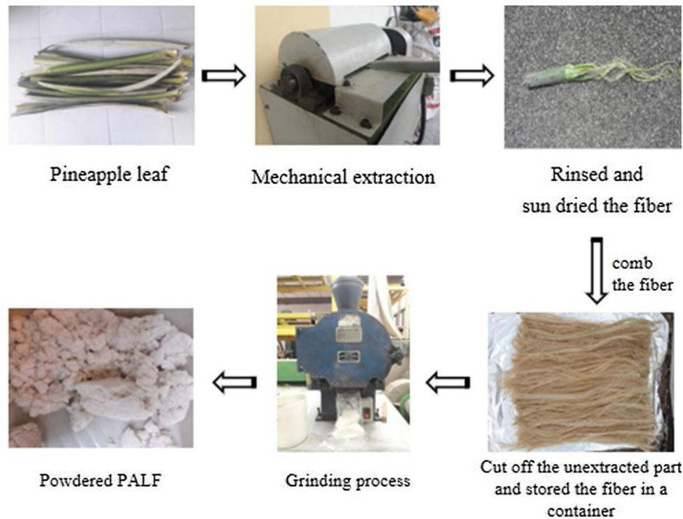
Fig. 1 – Material preparation process.
