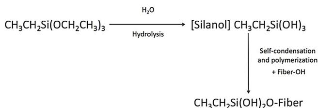
**Fig. 6 – Possible Silane reaction with fiber surface.**
