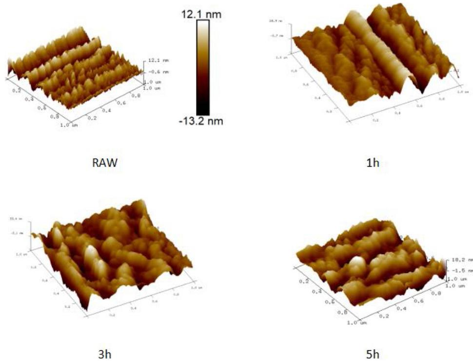
**Fig. 12 – 3-Dimensional presentation of the fiber surface texture.**
