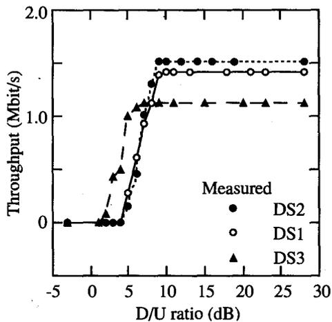
Fig. 3 Measured throughput of the DS systems with an FH1 disturbance source.
