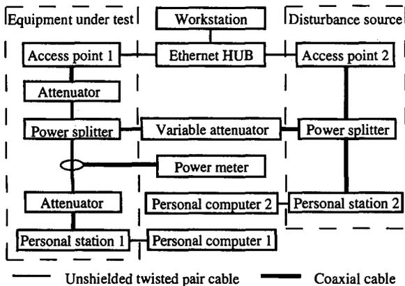
Fig. 1 Configuration for measuring interference characteristics.
