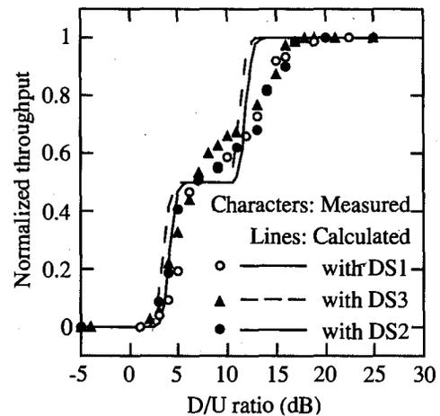
Fig. 10 Measured and calculated throughput of the FH system with a DS1, DS2, or DS3 disturbance source.
