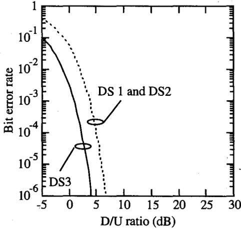
Fig. 6 Calculated bit error rates of the DS systems with an FH1 disturbance source.
