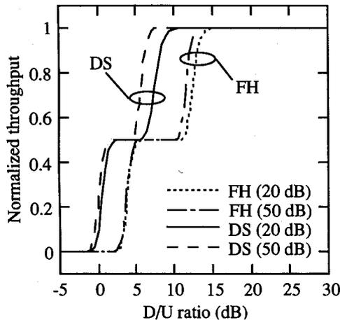
**Fig. 11** Interference characteristics between DS and FH systems based on IEEE 802.11.
