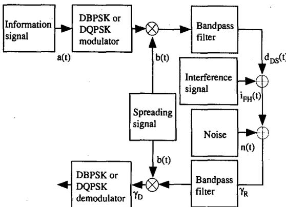
Fig. 5 Model used to simulate the DS systems.
