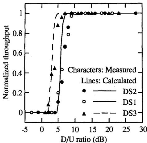
Fig. 9 Measured and calculated throughput of the DS systems with an FH1 disturbance source.
