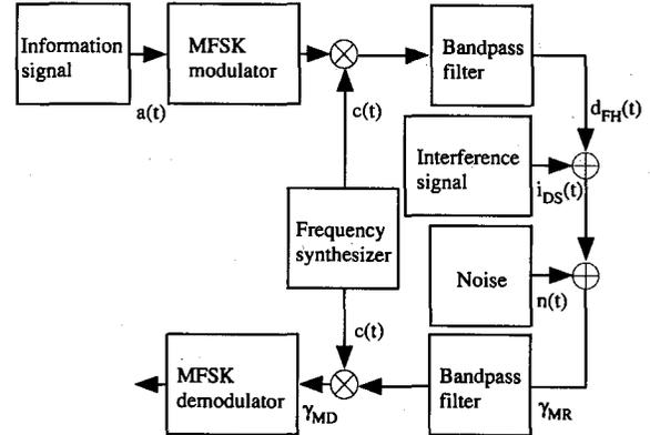
Fig. 7 Model used to simulate the FH system.
