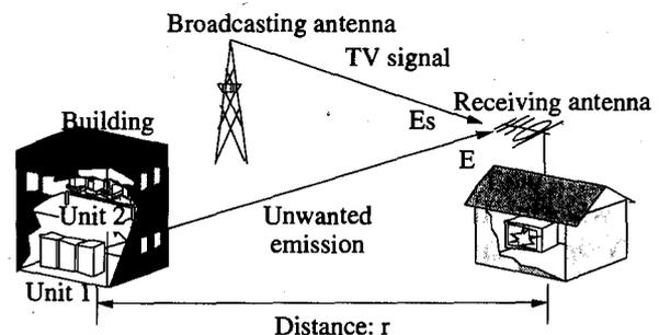
Fig. 1 Disturbance mechanism caused by emission.
