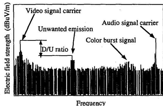
Fig. 2 Spectrum model of TV signal and unwanted emission.
