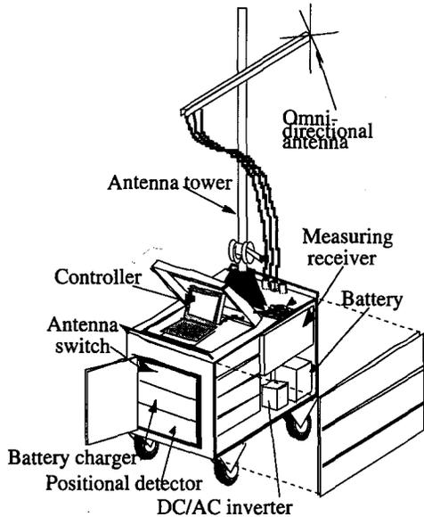
Fig. 4 Measuring system.
