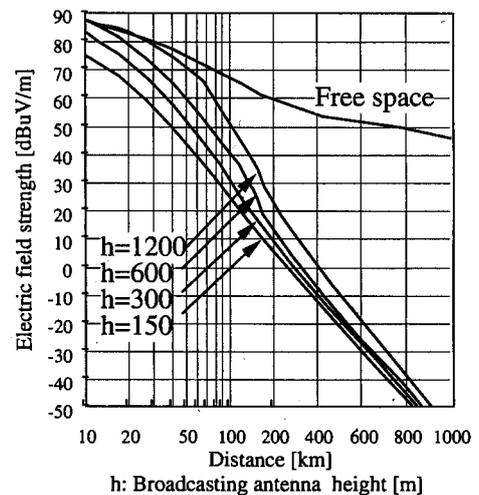
Fig. 7 Propagation of TV signals at  $E_{ep} = 1 \text{ kW}$ .
