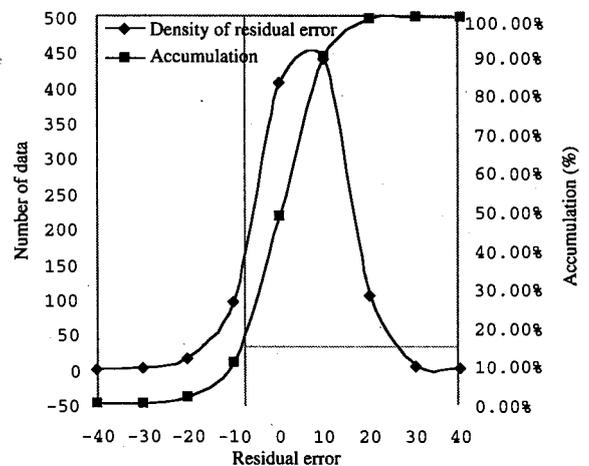
Fig. 6 Residual error distribution and accumulation.
