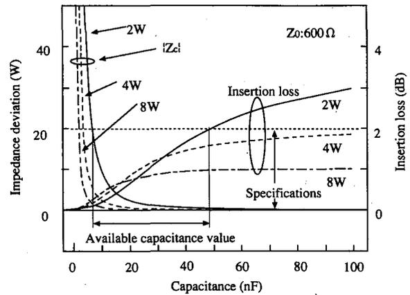
(a) Absolute value of common-mode impedance vs. insertion loss
