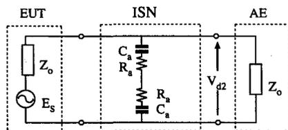
Fig. 7 Equivalent circuit of ISN for differential mode current.
