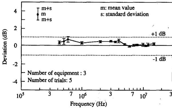
Fig. 15 Measurement deviation between two types of four-wire ISN.
