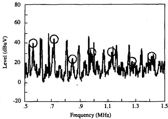
Fig. 3 Disturbance voltage measured by two 2W ISN.
