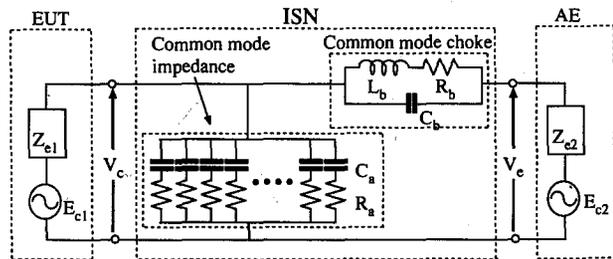
Fig. 6 Equivalent circuit of ISN for common mode current.
