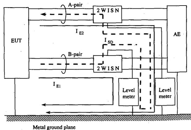
**Fig. 2** Equivalent circuit when two 2W ISN are used to measure disturbance voltage at telecommunication ports with 4W cable.
