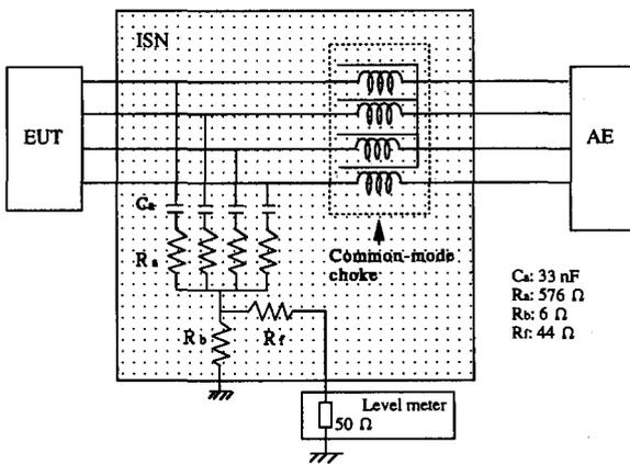
Fig. 13 Configuration of four-wire ISN.
