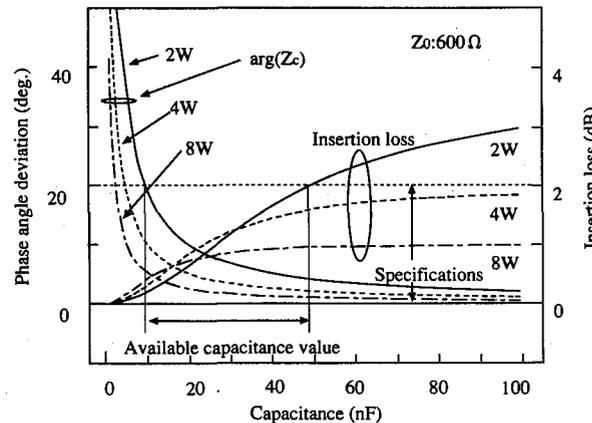
(b) Phase angle of common-mode impedance vs. insertion loss
