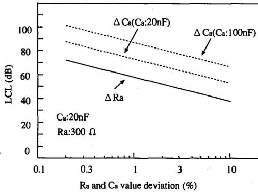
Fig. 10 Calculated result of longitudinal conversion loss.
