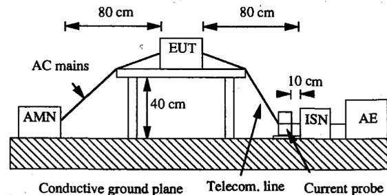
Fig. 14 Layout for measuring disturbances at telecommunication ports.
