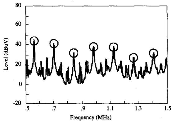
Fig. 4 Disturbance voltage measured by newly developed 4W ISN.
