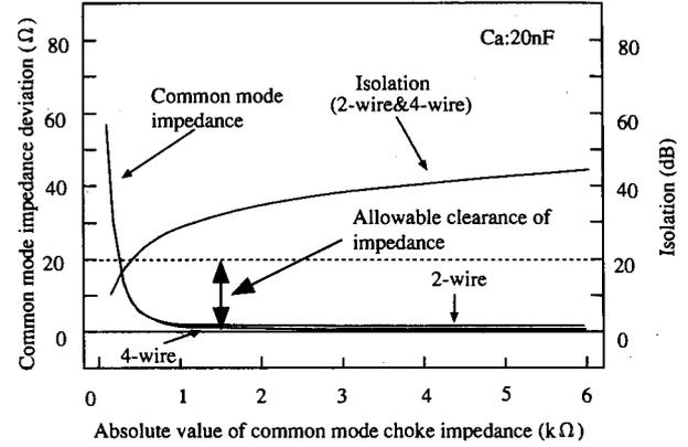
Fig. 9 Relation between common mode impedance and impedance of common mode choke.
