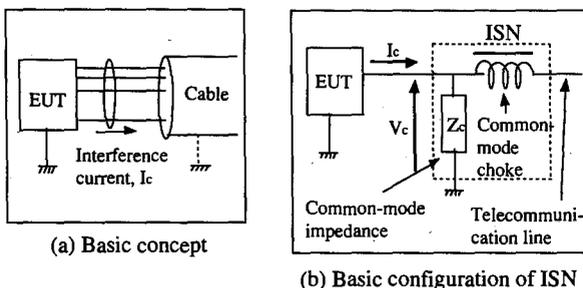
**Fig. 1** Basic concept and configuration of ISN.
