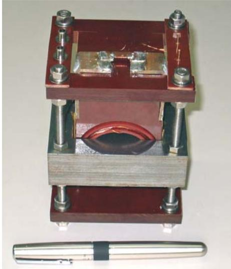
**Figure 1.** Image of the superconducting transformer. The size is about 80 mm × 100 mm × 140 mm and the weight is about 1.5 kg. The copper bridge on the upper side is used as a shunt for measuring the output current.
