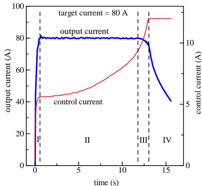
**Figure 2.** Result of the controlled output current (thick line) under the variation of the control current (thin line).
