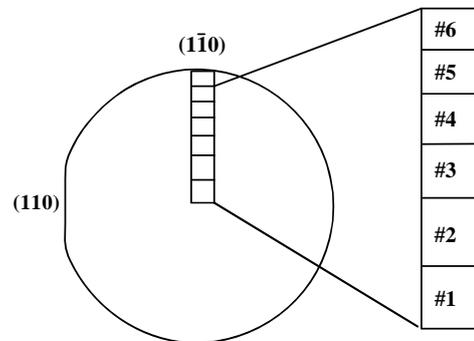
**Fig. 1:** Position of the six pieces of the GaAs/Al<sub>x</sub>Ga<sub>1-x</sub>As QW's on the 2-inch wafer numbered from #1 at the center to #6 at the edge.
