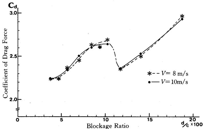
Fig. 2 Coefficient of Drag Force in Various Blockage Ratio with Diameter of End Plates of 450mm
