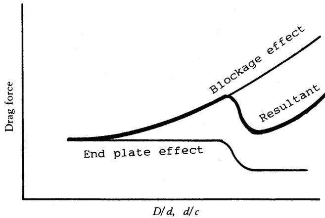
Fig. 6 Resultant Effects of Blockage and End Plates Effects
