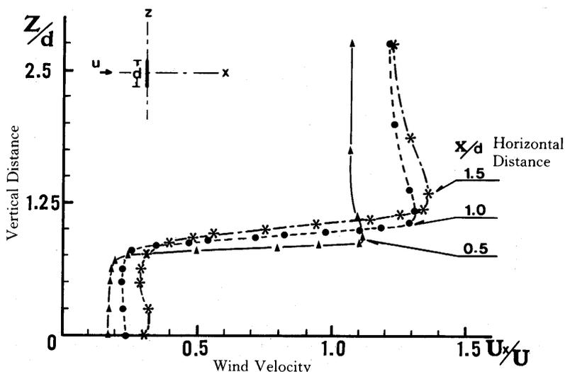
Fig. 8 Horizontal Component of Wind Velocity Profile in the Wake of End Plate Diameter Ratio ( $D/d=4$ )
