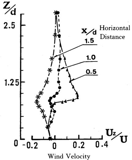
Fig. 11 Vertical Component of Wind Velocity Profile in the Wake of End Plate Diameter Ratio  $D/d=10$
