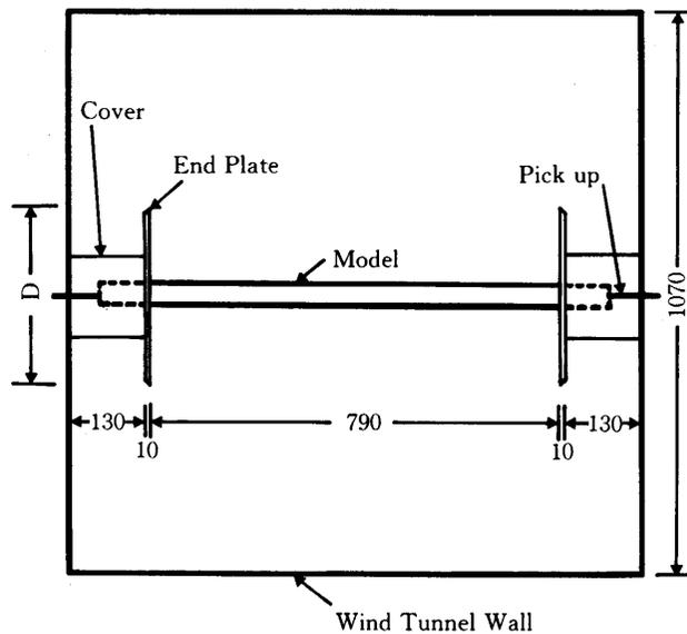
Fig. 1 Model and Mounting System of Wind Tunnel
