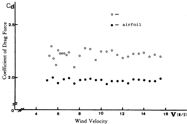
Fig. 4 Coefficient of Drag Force due to Circular Shaped and Aerofoil Cover of Support
