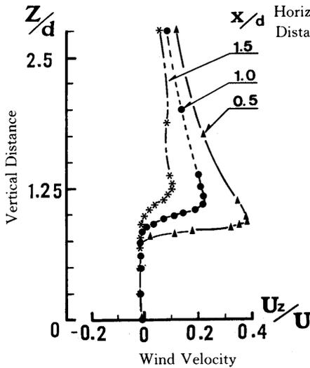
Fig. 10 Vertical Component of Wind Velocity Profile in the Wake of End Plate Diameter Ratio  $D/d=4$
