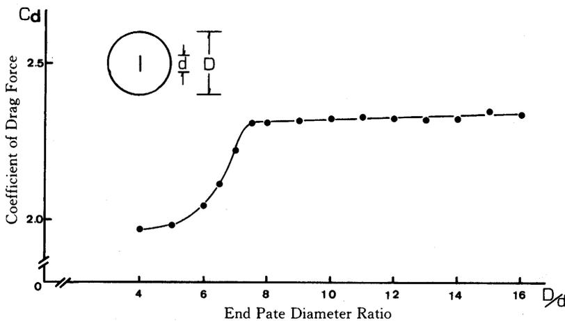
Fig. 5 Coefficient of Drag Force in various End Plate Diameter Ratio to Model Width
