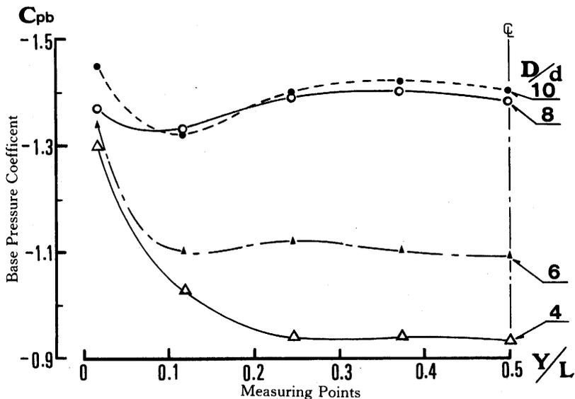
Fig. 7 Base Pressure Distribution for Various End Plate Ratio ( $D/d=4, 6, 8, 10$ )
