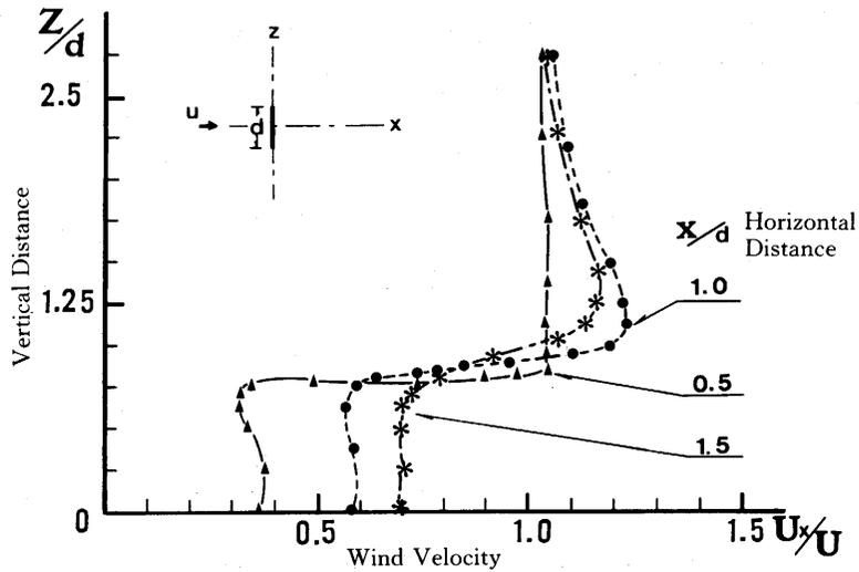
Fig. 9 Horizontal Component of Wind Velocity Profile in the Wake of End Plate Diameter Ratio ( $D/d=10$ )
