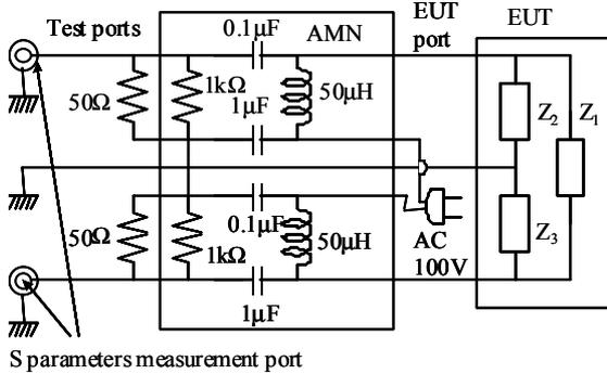
Figure 4. Measurement system of electronic appliance
