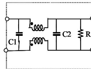
Figure 12. Circuit of power line filter
