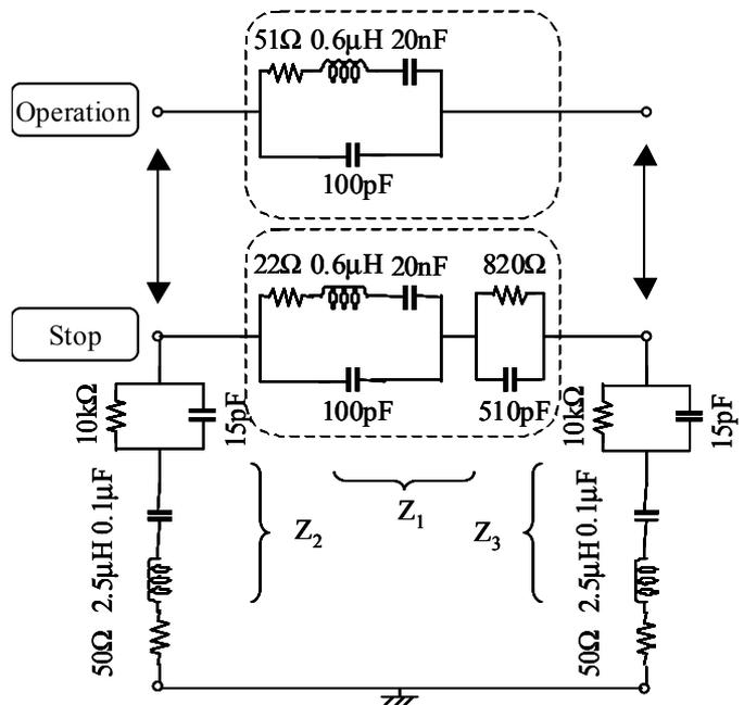
Figure 8. Equivalent circuit of electric fan
