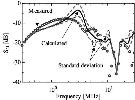
Figure 11.  $S_{21}$  when the state of appliance changes
