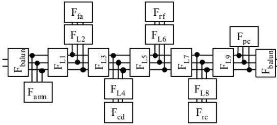
Figure 2. Analysis model of AC mains line presented by four-port and two-port networks
