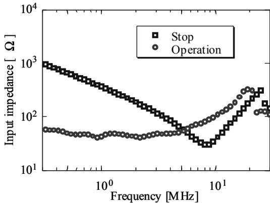
Figure 6. Example of measured input impedance (electric fan)
