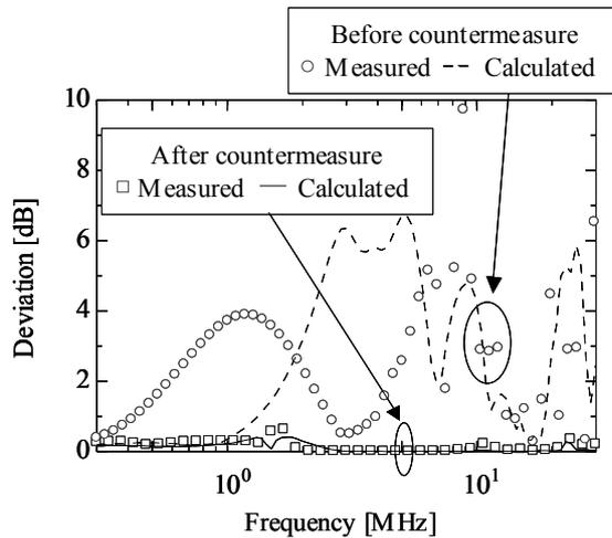
Figure 14. Deviation of S21 value when AC mains line condition are changed
