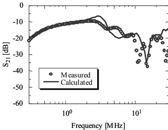
Figure 10. Measurement and calculated values of  $S_{21}$  from AMN to PC when all appliances are Operating
