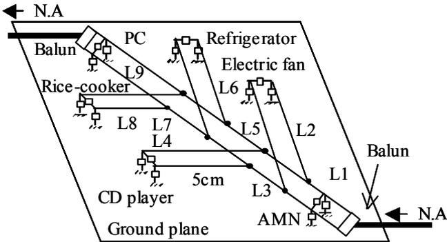
Figure 9. Experimental set-up for measuring  $S_{21}$
