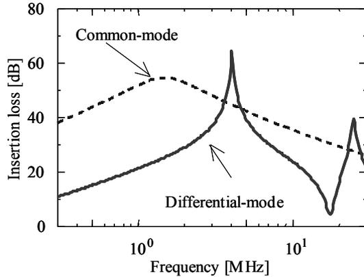
Figure 13. Frequency characteristics of common-mode choke coil
