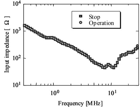
Figure 5. Example of measured input impedance (CD player)
