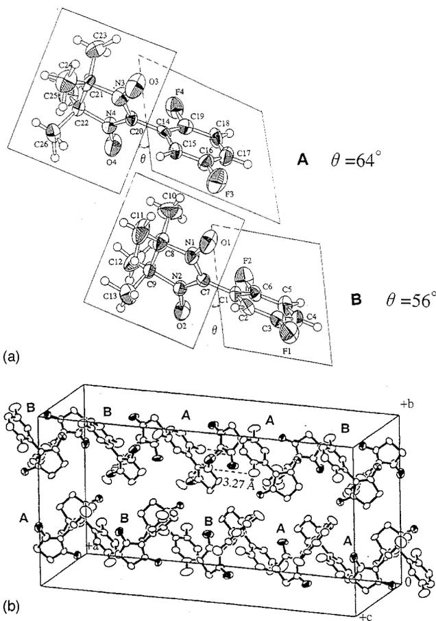
FIG. 2. (a) Molecular structure of 2,5-DFPNN. (b) The schematic molecular stacking in the unit cell. The unit cell consists of two rotational isomers (A and B), which are stacked as -A-A-B-B-A-A- along the  $a$  axis.
