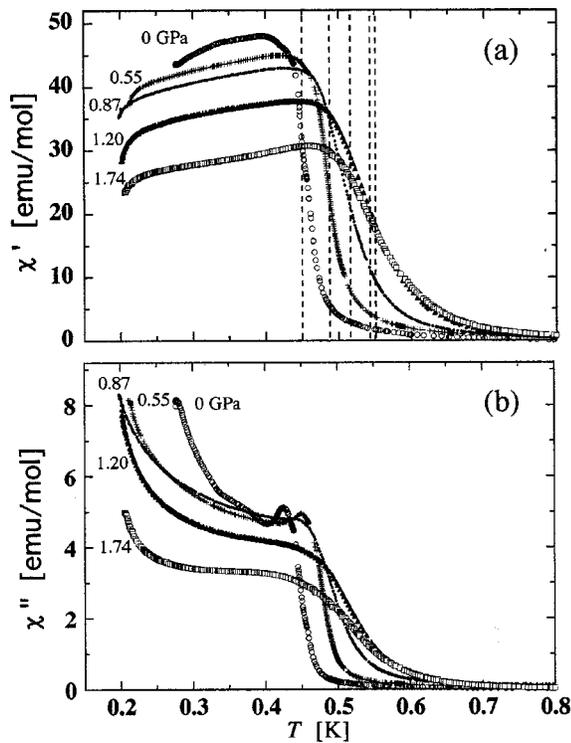
FIG. 5. Pressure dependences of in-phase component  $\chi'$  (a) and out-of-phase one  $\chi''$  (b) of ac magnetic susceptibility for 2,5-DFPNN under hydrostatic pressure up to  $P = 1.74$  GPa. The transition temperature ( $T_c$ ) to the ferromagnetic long-range order at each pressure is shown by dotted line, and it shifts toward high temperatures with increasing pressure.
