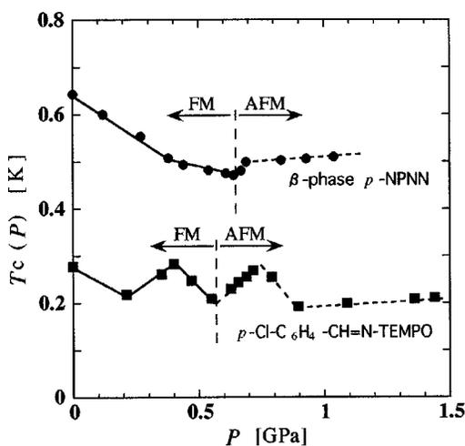
FIG. 1. Pressure dependence of transition temperature ( $T_c$ ) in two typical organic radical ferromagnets, the  $\beta$  phase of  $p$ -NPNN [ $T_c(P=0)=0.61$  K] (Refs. 7–9) and  $p$ -Cl-C<sub>6</sub>H<sub>4</sub>-CH=N-TEMPO [ $T_c(P=0)=0.28$  K] (Ref. 10). The solid and dotted lines stand for the ferromagnetic (FM) and antiferromagnetic (AFM) regions, respectively.
