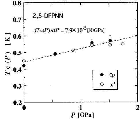
FIG. 4. Pressure dependence of the ferromagnetic transition temperature ( $T_c$ ) of 2,5-DFPNN estimated from the heat capacity  $C_p$  (●) and the in-phase ac susceptibility  $\chi'$  measurements (○). The dotted line expresses  $T_c(P) = 7.9 \times 10^{-2} P + 4.5 \times 10^{-1}$ .
