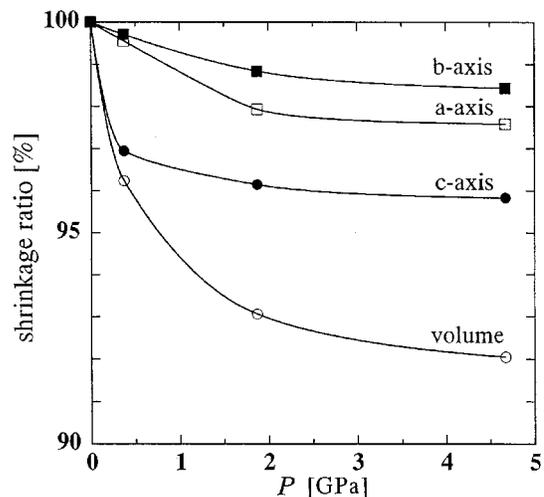
FIG. 7. Pressure dependences of the lattice constants ( $a$ ,  $b$ , and  $c$ ) and the volume of unit cell ( $V$ ) of 2,5-DFPNN. The solid curves are the guides for the eye.
