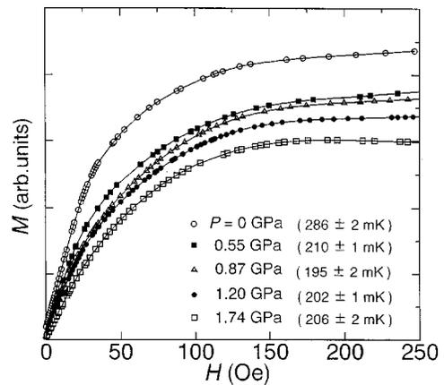
FIG. 6. Pressure dependence of the magnetization ( $M$ ) curve of 2,5-DFPNN up to magnetic field ( $H$ ) 250 Oe in the hydrostatic pressure region below  $P = 1.74$  GPa. Each measurement was performed at the lowest temperature in each measurement, which was sufficiently below each  $T_c$ .
