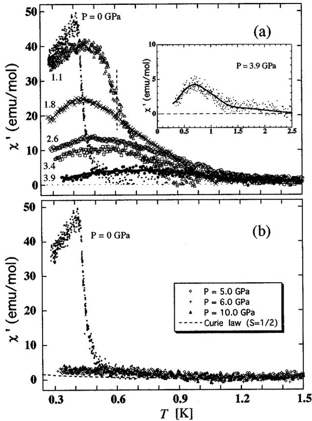
FIG. 8. Pressure dependence of in-phase ac magnetic susceptibility ( $\chi'$ ) of 2,5-DFPNN under nonhydrostatic pressure: (a) for  $P \leq 3.9$  GPa, and (b) for  $P = 0, 5.0, 6.0,$  and  $10.0$  GPa. The dotted line in (a) shows the imaginary  $T_c$  at  $P = 1.1$  GPa. The dotted curve in (b) expresses the Curie's law for  $S = \frac{1}{2}$ .
