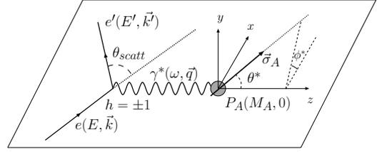
FIG. 1. Spin-dependent inclusive electron scattering from a polarized target. The target spin angles  $\theta^*$  and  $\phi^*$  are defined with respect to the three-momentum transfer vector  $\mathbf{q}$ .
