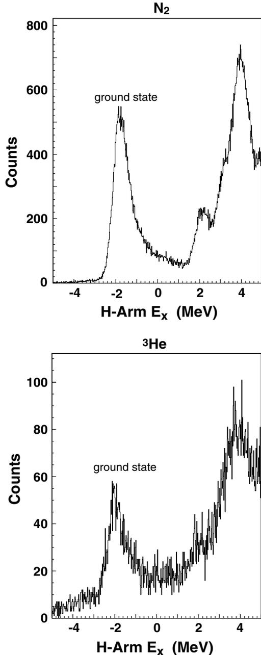
FIG. 3. Raw yields measured with the right-arm spectrometer in the region of the  $N_2$  elastic peak using the  $N_2$  reference cell (upper panel) and the  $^3\text{He}$  target (lower panel) as a function of excitation energy  $E_x$ . The leftmost peak represents the  $N_2$  ground state; other peaks are related to excited states of  $N_2$ .
