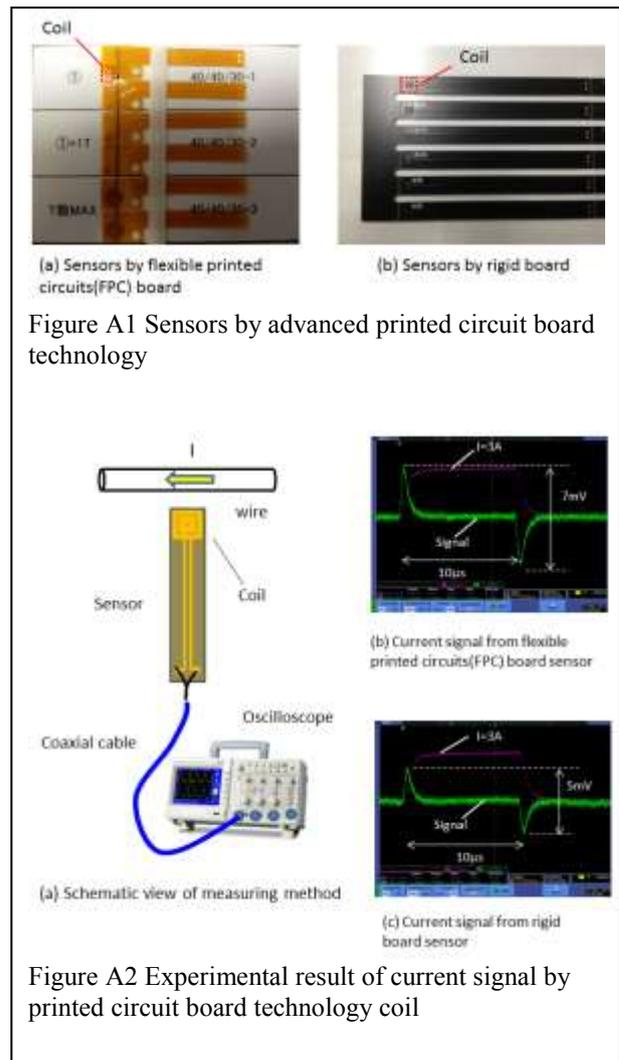
Figure A1 Sensors by advanced printed circuit board technology
