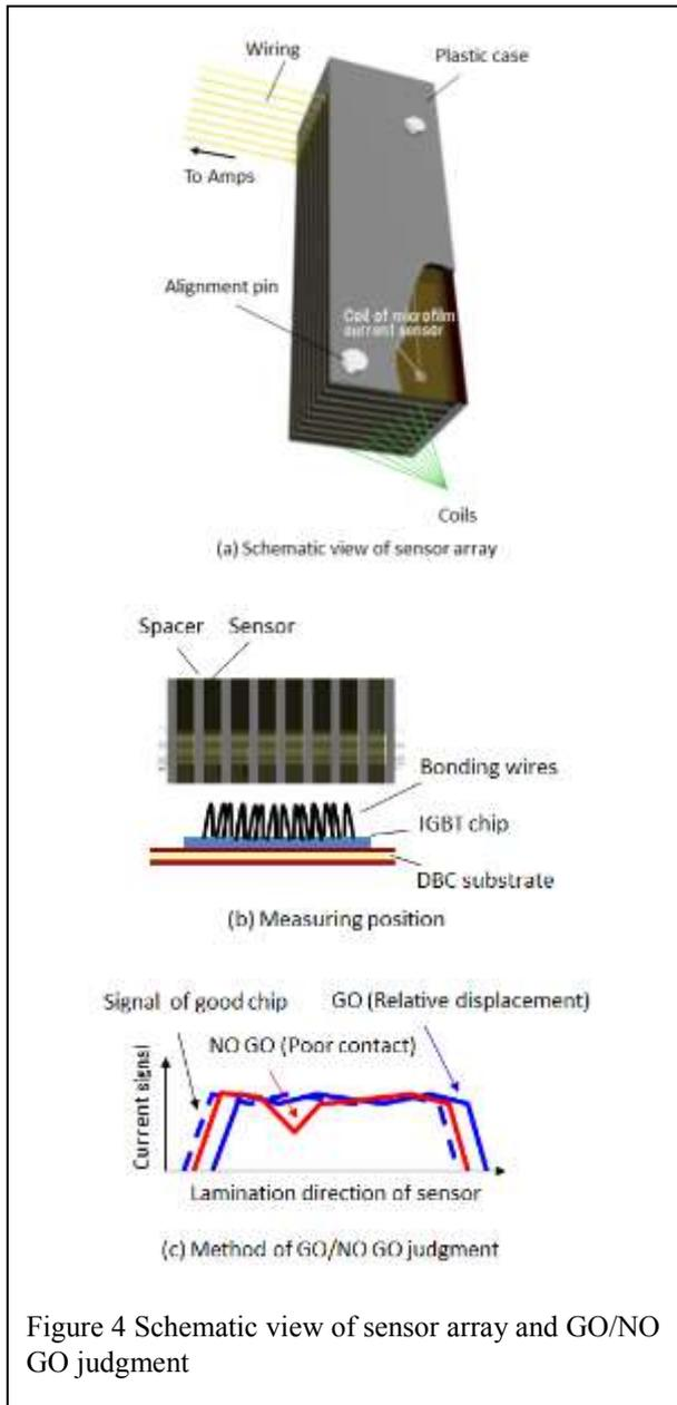
Figure 4 Schematic view of sensor array and GO/NO GO judgment
