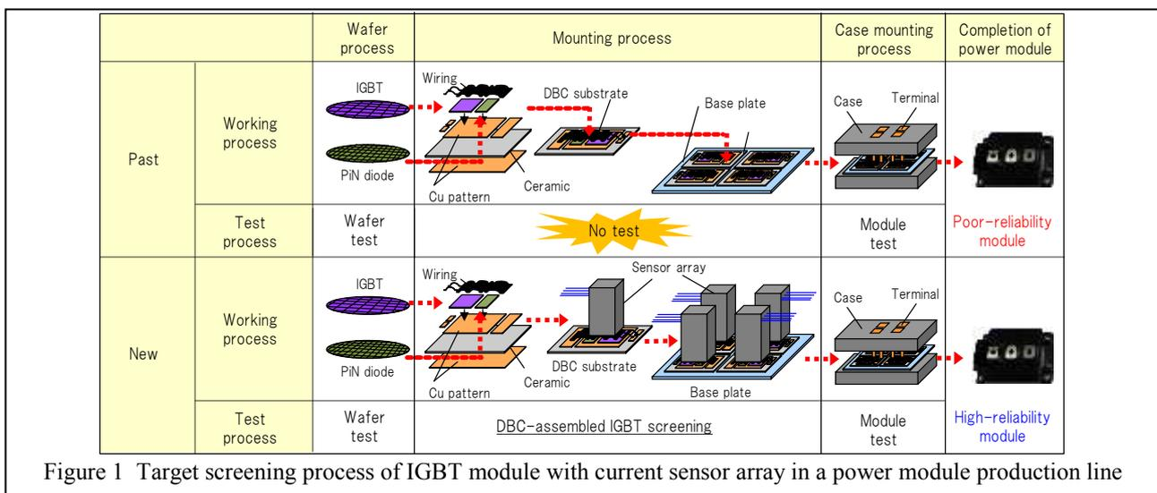
Figure 1 Target screening process of IGBT module with current sensor array in a power module production line
