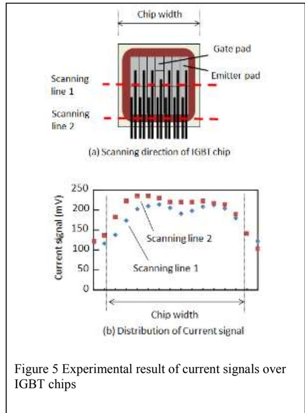
Figure 5 Experimental result of current signals over IGBT chips
