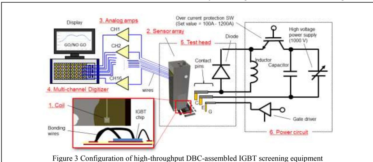
Figure 3 Configuration of high-throughput DBC-assembled IGBT screening equipment
