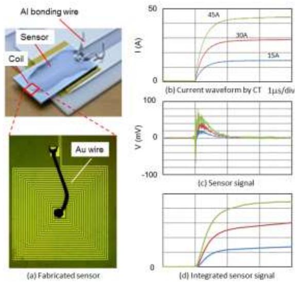
Figure A4 Experimental result of current signal by semiconductor process technology coil (L/S=10µm)
