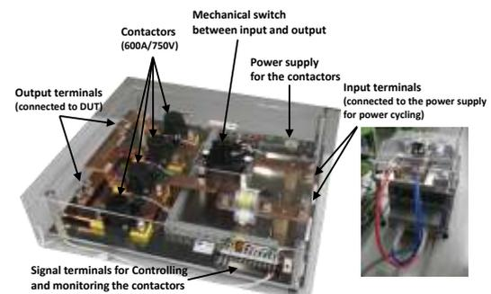
**Figure 4** Switching system constructed by TTL control contactors
