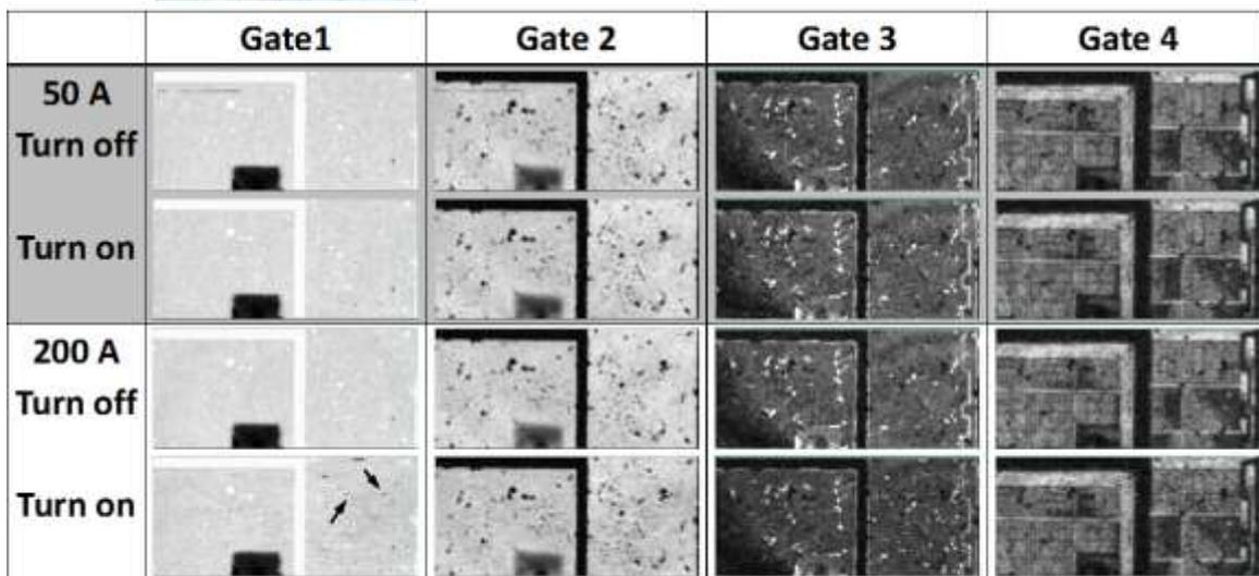
**Figure 6** Internal SAT images of the DUT obtained under the different load current. The biased high-side chip is observed in the right side region of each image. The inside photograph is upset the top and bottom to adjust to these SAT images observed from the base plate substrate. A rectangular shadow in the bottom center is a shadow of adhesive tape to settle the temperature sensor.
