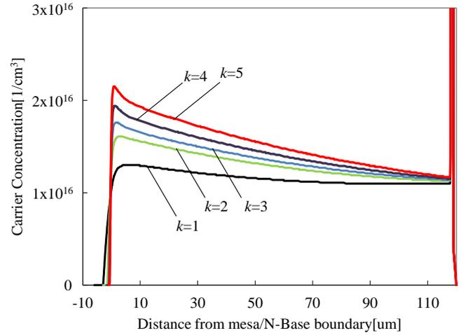
Fig. 5. Calculated carrier distribution in N-Base region for scaling factor  $k=1$  to 5. The zero point of horizontal scale is set to mesa/N-Base boundary. Cathode side carrier concentration is increased by scale down.
