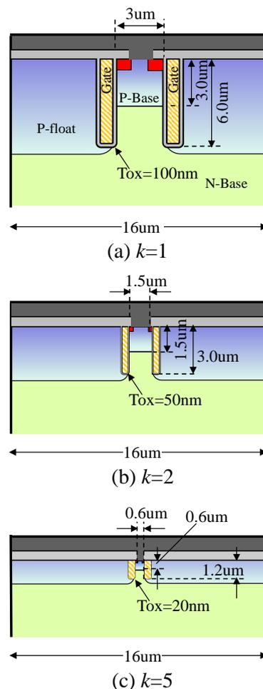
Fig. 1. Concept of trench gate IGBT scaling rule.
