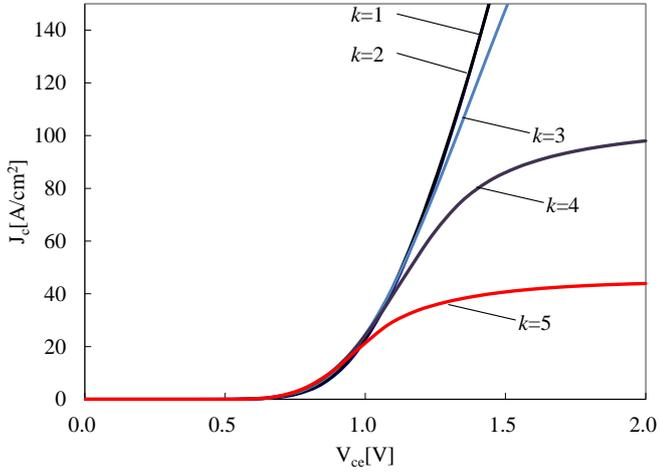
Fig. 3. Calculated  $I_c$ - $V_c$  characteristics of scaled devices with scaled electric field in gate oxide as  $E_{ox}'=E_{ox}/k$ .  $k=1$  and 2 show good agreement but more scaled devices show lower saturation current.
