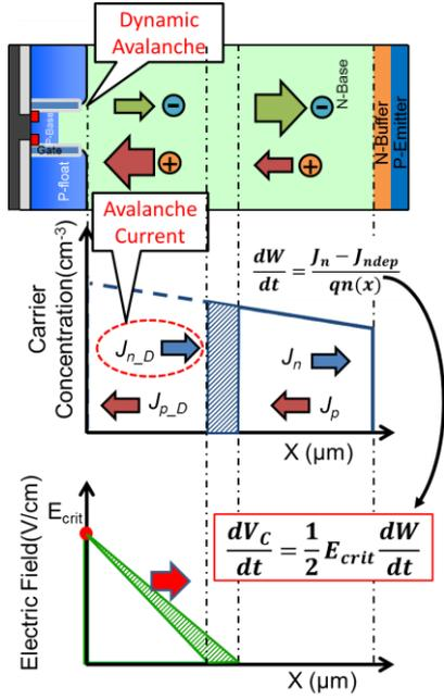
Fig. 5. Turn-off mechanism after dynamic avalanche the formulation.
