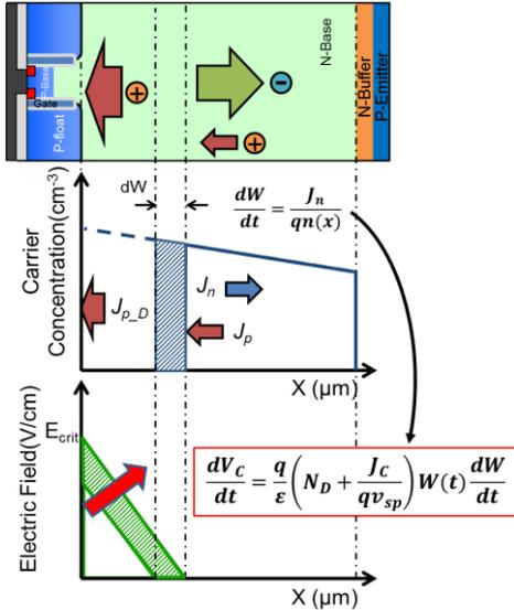
Fig. 4. Turn-off mechanism before dynamic avalanche and the formulation.
