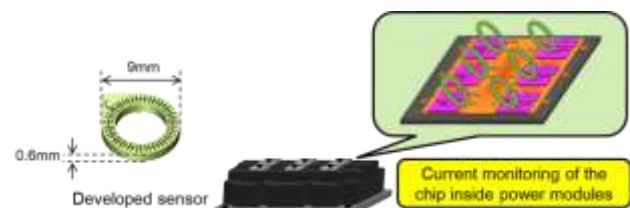
Figure 2 Application example of the power modules of the developed sensor
