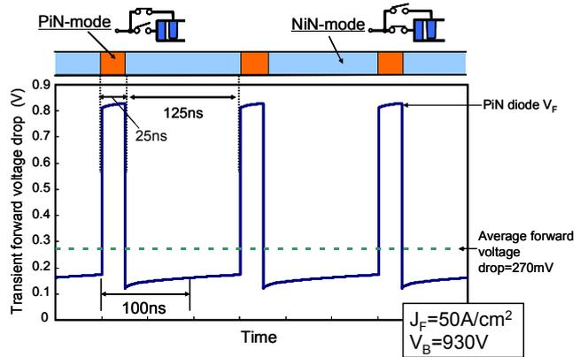
Figure 4. TCAD simulation result of transient forward voltage drop of proposed diode (the diode has  $V_B=930 \text{ V}$ ). The forward voltage is below 200 mV during NiN-mode since no PN junction appears along the current path, while the 0.8 V voltage drop appears during PiN-mode. The average value of forward voltage drop is as low as 270 mV.
