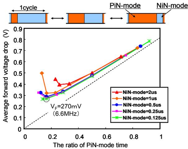
Figure 6. TCAD simulation results of average forward voltage drop for the diode with the pulsed carrier injection as a function of PiN-mode time in the cycle. Frequencies of the pulse cycle are also described in the figure. Increasing the pulse frequency, the optimum average forward voltage drop decreases
