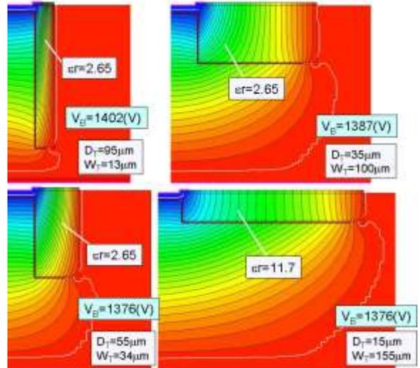
Fig.9 Practical trench termination structures for each depth.
