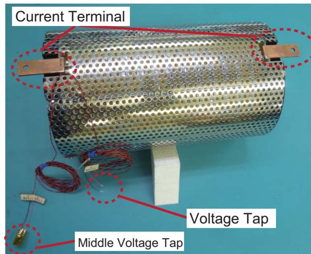
**FIGURE 4.** Bi-2223 superconducting magnet made from 28 double-pancake coils.
