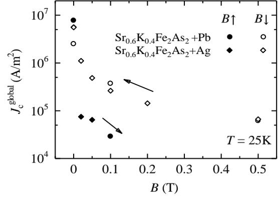
Fig. 5. Magnetic field dependence of global  $J_c$  in (Sr,K)-122 samples with 10wt.% Pb or Ag addition. The close and open symbols denote the processes of magnetic field increasing and decreasing, respectively.
