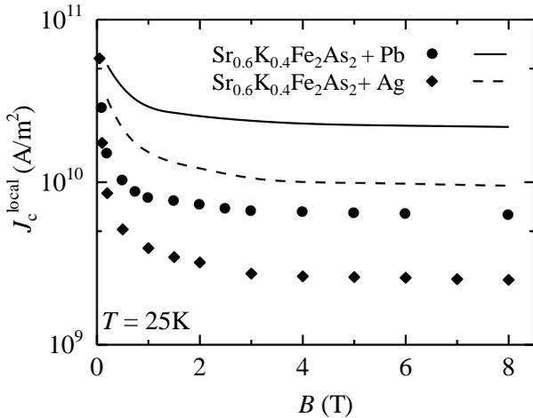
Fig. 4. Magnetic field dependence of local  $J_c$  in (Sr,K)-122 samples with 10wt.% Pb or Ag addition. The corrected curves in which the distribution of the grain size are shown by solid ((Sr,K)-122 + Pb) and dashed ((Sr,K)-122 + Ag) lines, respectively.
