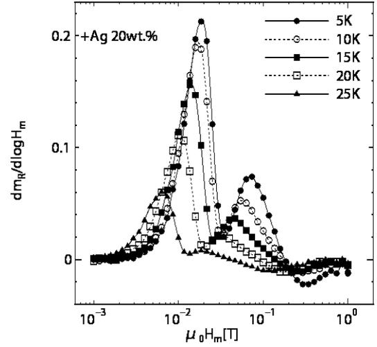
Fig. 1. Derivative of remnant magnetic moment as a function of maximum external magnetic field at various temperatures in sample with Ag 20wt.% added.
