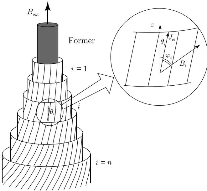
Fig. 3. Schematic illustration of winding structure of coated conductors in inner conductor. The angle  $\theta_i$  for the current is measured from the cable axis, and  $\varphi_i$  is the angle between the current and magnetic field. The axial magnetic field produced by the outside shield conductor is  $B_{\text{ext}}$ .
