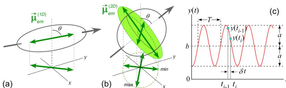
Fig. 2. Conceptual detection schemes for (a) linearly-polarized emission by a linear emitting transition dipole and (b) plane-polarized emission from a twofold degenerate dipole. Sample  $xy$ -plane is indicated. The graph in (c) indicates the time-trace pattern expected to be obtained by polarization modulations and the figure includes some of the parameters used in the following analysis..
