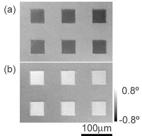
**Fig. 3** Kerr rotation images of patterned YBFGO thin films measured with a wavelength of 500 nm and magnetic field of (a) 750 and (b) -750 Oe. Dimension of a dot is  $50 \mu\text{m} \times 50 \mu\text{m}$  and thickness of 400 nm.
