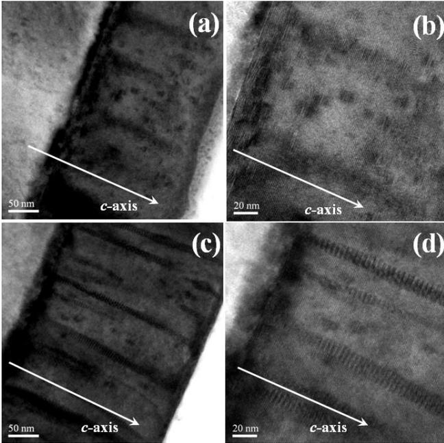
**FIG. 1** Cross-sectional transmission electron micrographs of YBCO+Y211 film (a), (b) and YBCO+BSO2%+Y211 film (c), (d) at different magnifications. The formation of nanoparticles in both the cases and that of nanocolumns in sample with hybrid APCs can be observed.
