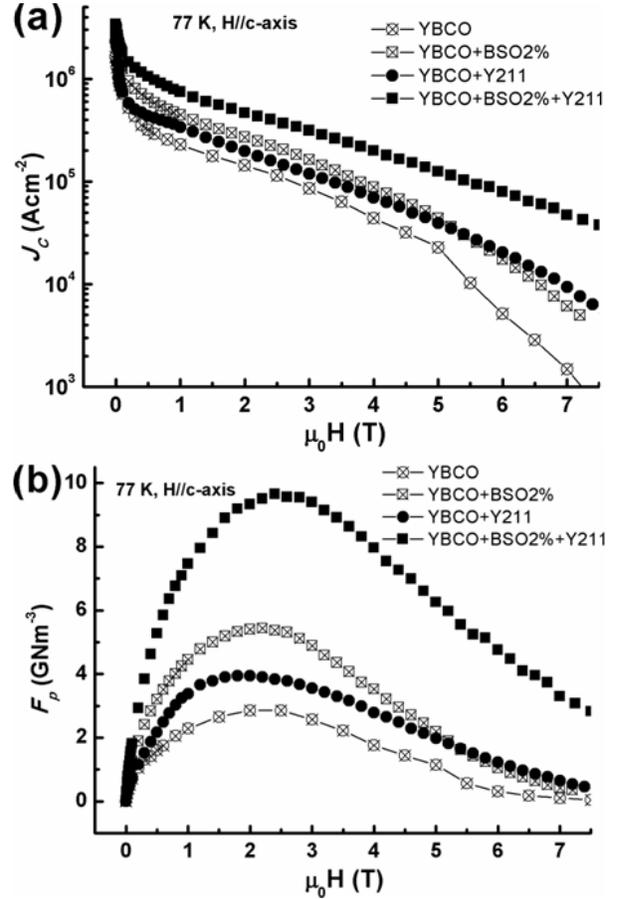
**FIG. 2** Variation of  $J_c$  (a) and  $F_p$  (b) with applied magnetic field for YBCO, YBCO+BSO2%, YBCO+Y211 and YBCO+BSO2%+Y211 at 77 K.
