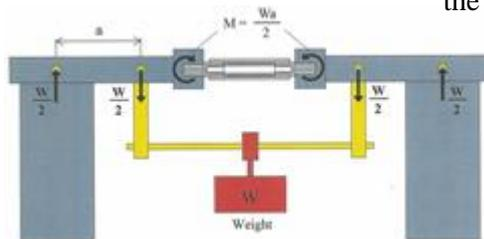
Figure 11 Schematic view of rotating bending machine
