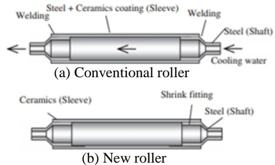
Figure 2 Roller structure
