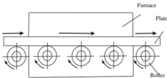
Figure 1 Layout of rollers in heating furnace
