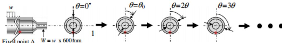
Figure 5 The rotation of the roller replaced by the shifted load at the interval of the load shift angle  $\theta_0$ . When  $\theta = 0^\circ$  the number of cycle  $N = 0$ , and when  $\theta = 360^\circ$  the number of cycle  $N = 1$ .
