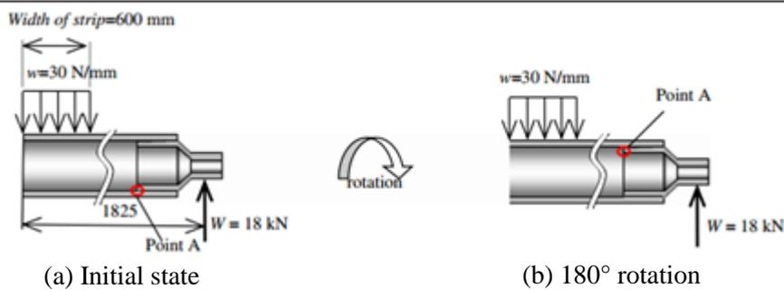
Figure 4 Dimensions and loading condition of new roller
