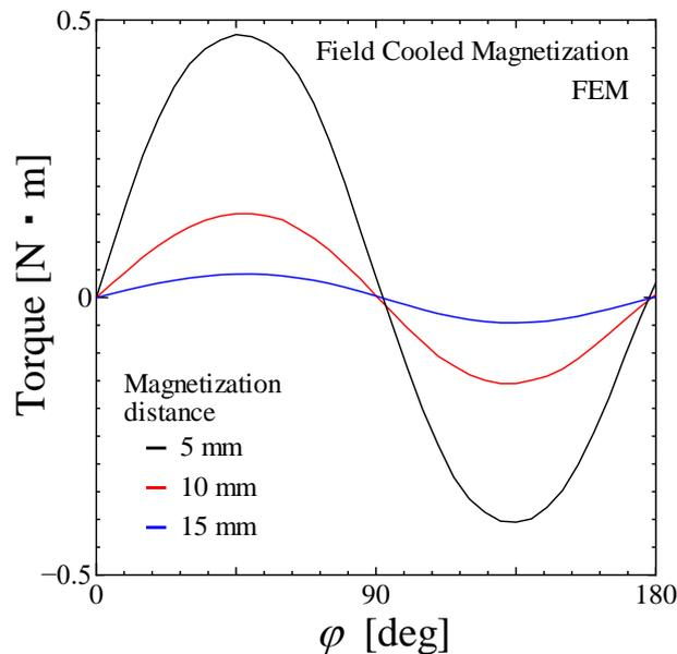
**Figure 7.** Rotational torque as a function of angle with various initial magnetization distance.
