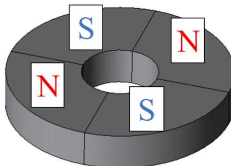
**Figure 2.** 4-pole magnet used in the SUAM.
