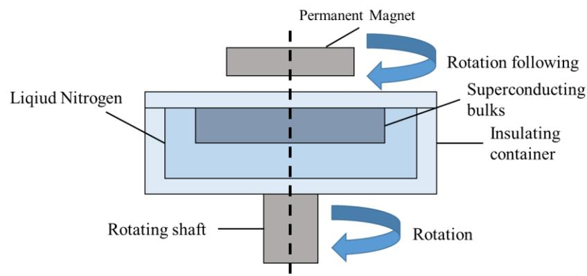
**Figure 1.** Schematic illustration of SUAM (Superconductive Assisted Machine).
