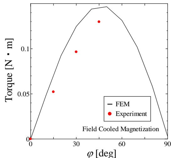
**Figure 6.** Rotational torque as a function of angle when initial magnetization distance is 10 mm.
