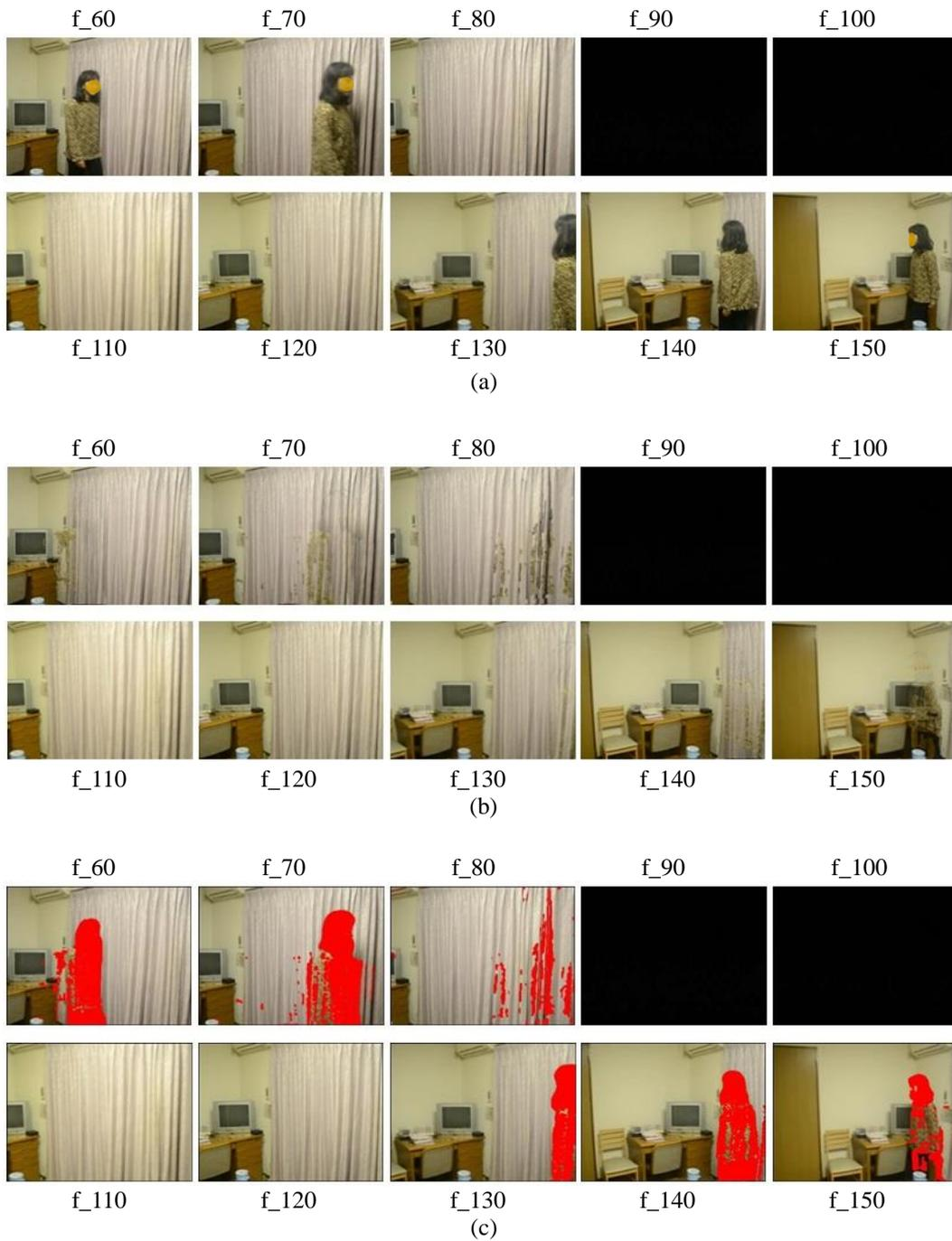
**Fig. 3.** Foreground object detection in the case of large illumination change: (a) Part of the original image sequence, (b) the background model employing Eqs.(3,4), (c) the result of moving object (foreground pixels) detection: Foreground pixels are indicated by red.
