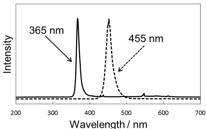
Fig. 1 Emission spectrum of the LED (365 or 455 nm)
