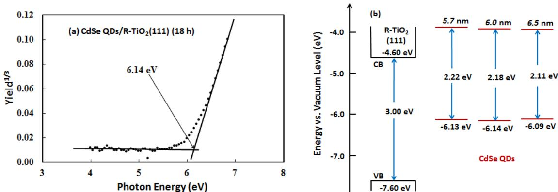
**Figure 4.** (a) Photoelectron yield spectrum of CdSe quantum dots adsorbed on the (111) surface of single crystal R-TiO<sub>2</sub>. (b) alignment of energy levels.
