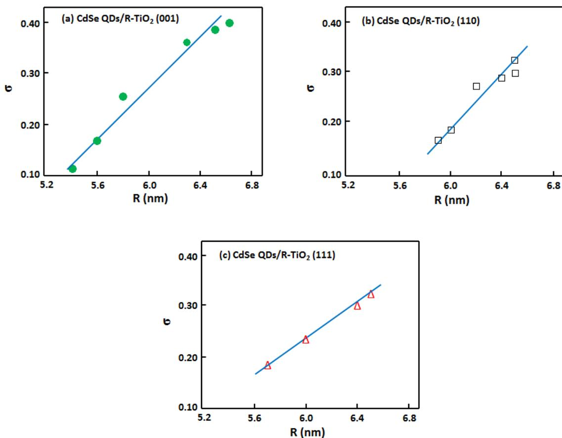
**Figure 3.** Dependence of steepness parameter,  $\sigma$ , on the average diameter,  $R$ , of CdSe quantum dots adsorbed on the (a) (001), (b) (110), and (c) (111) surfaces of single crystal R-TiO<sub>2</sub>.
