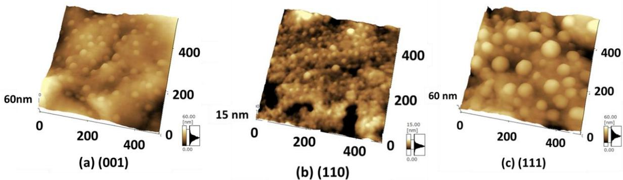
**Figure 1.** AFM images of CdSe quantum dots adsorbed on the (a) (001), (b) (110), and (c) (111) surfaces of single crystal of R-TiO<sub>2</sub> (adsorption temperature 10°C; adsorption time, 4 h).
