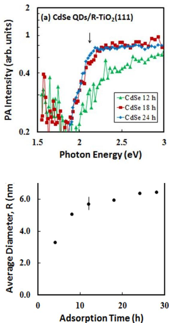
**Figure 2.** (a) Photoacoustic spectra for CdSe quantum dots adsorbed on the (111) surface of single crystal R-TiO<sub>2</sub>. (b) Dependence of average diameter,  $R$ , on adsorption time.
