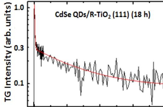
**Figure 6.** Transient grating response for CdSe quantum dots adsorbed on the (111) surface of single crystal R-TiO<sub>2</sub> (adsorption time, 18 h).
