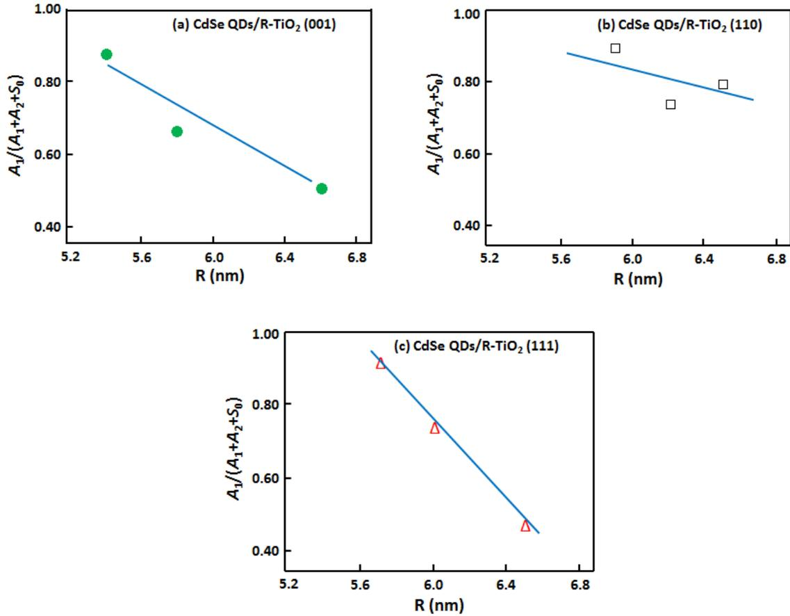
**Figure 7.** Dependence of the relative component of  $A_1/(A_1 + A_2 + S_0)$  on the average diameter,  $R$ , of CdSe quantum dots adsorbed on the (a) (001), (b) (110), and (c) (111) surfaces of single crystal R-TiO<sub>2</sub>.
