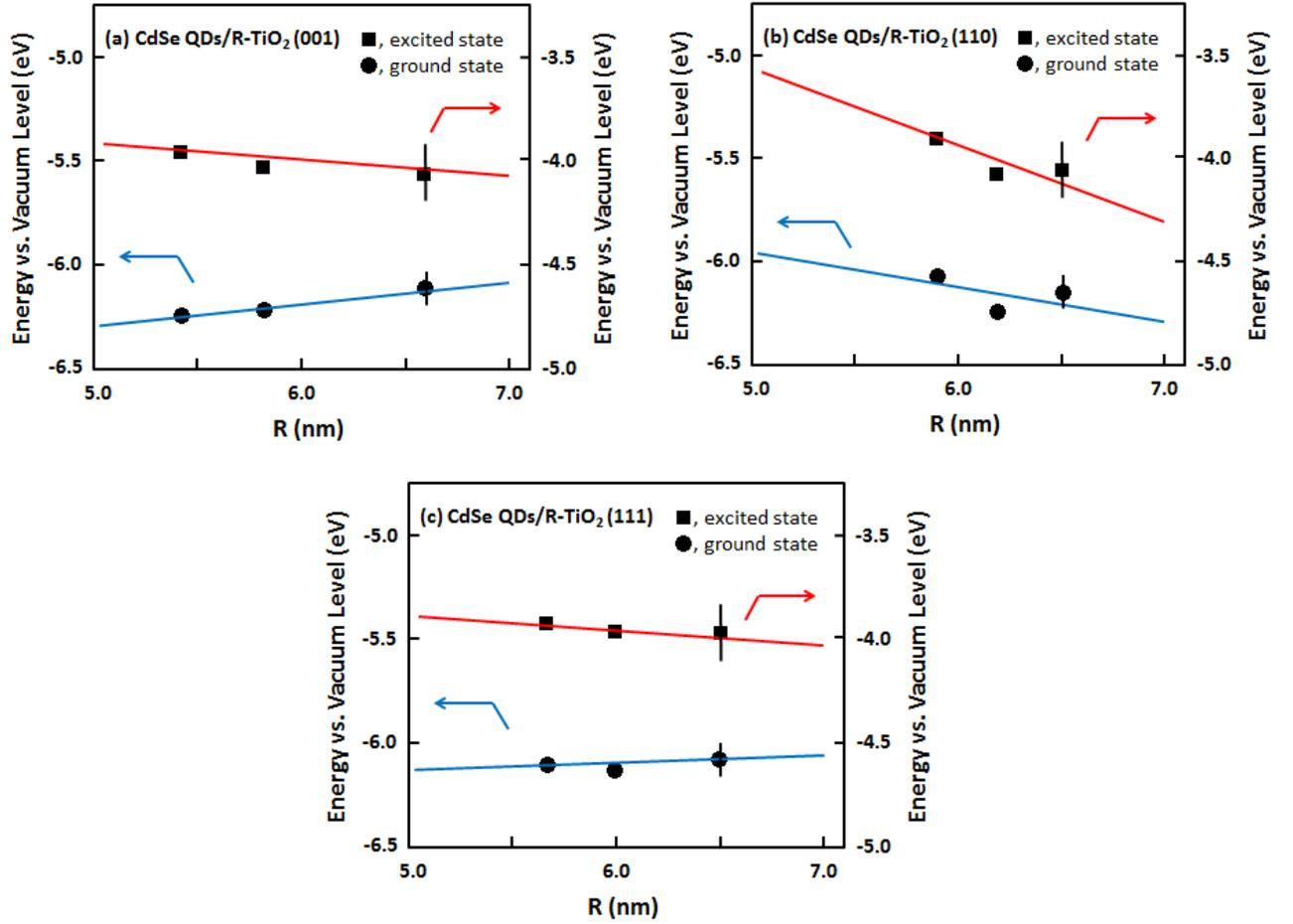
**Figure 5.** Dependence of ground state and excited state energy levels of CdSe quantum dots on average diameter,  $R$ , adsorbed on the (a) (001), (b) (110), and (c) (111) surfaces of single crystal R-TiO<sub>2</sub>
