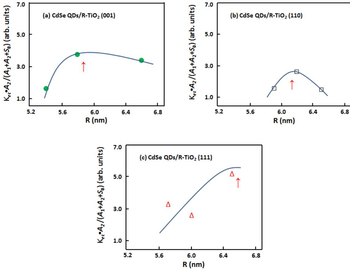
**Figure 10.** Dependence of the value of  $K_{et} \cdot A_2 / (A_1 + A_2 + S_0)$  on the average diameter,  $R$ , of CdSe quantum dots adsorbed on the (a) (001), (b) (110), and (c) (111) surfaces of single crystal R-TiO<sub>2</sub>.
