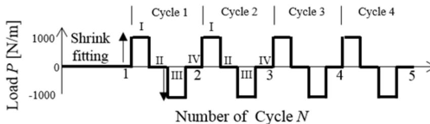
**Figure 5.** New alternate loading pattern with intervals.
