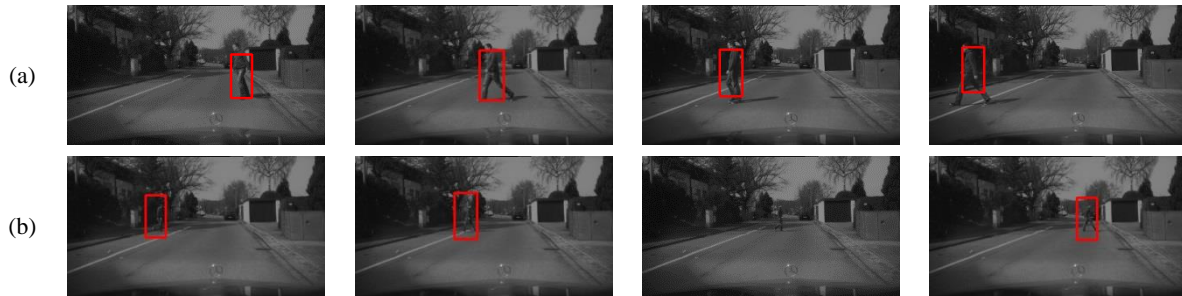
Figure 4. Detection results on videos: (a) Crossing from right to left, (b) crossing from left to right.
