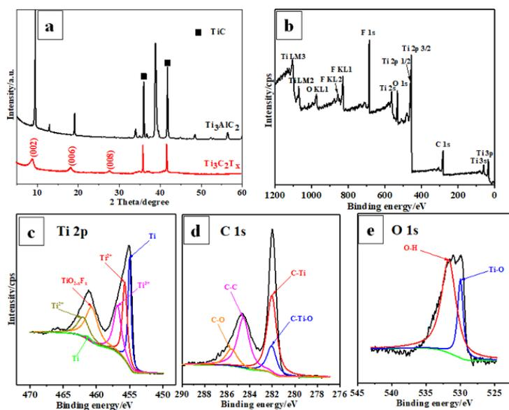
**Figure 1.** (a) XRD patterns of  $\text{Ti}_3\text{AlC}_2$  raw materials (black line) and sample after HF etching (red line), (b) XPS spectra of  $\text{Ti}_3\text{C}_2\text{Ti}_x$  sample and the high-resolution spectra of (c) Ti 2p, (d) C 1s and (e) O 1s.
