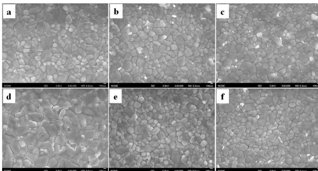
**Figure 2.** SEM images of the perovskite film with different amount of  $\text{Ti}_3\text{C}_2\text{Ti}_x$ -DMF additive: (a) 0 wt%, (b) 0.01 wt%, (c) 0.02 wt%, (d) 0.03 wt%, (e) 0.05 wt% and (f) 0.1 wt%.
