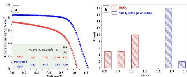
**Fig. 4** (a)  $J$ - $V$  curves of the champion PSCs based on bare or passivated SnO<sub>2</sub> ESL (inset table is the photovoltaic parameters); (b)  $V_{oc}$  distributions of two type PSCs (20 cells for each).
