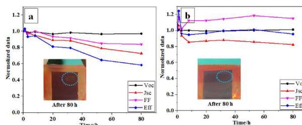
**Fig. 7** Normalized photovoltaic parameters of the (a) bare and (b) passivated SnO<sub>2</sub> ESL based unencapsulated CsPbI<sub>2</sub>Br<sub>2</sub> PSCs under continuously heating at 90 °C in air with the humidity of 60-70%. Inset are the photographs of the two kinds of PSCs after heating for 80 hours.
