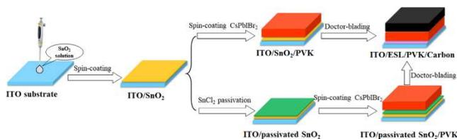
**Fig. 1** Fabrication process of all-inorganic PSCs with bare or passivated SnO<sub>2</sub> ESL.
