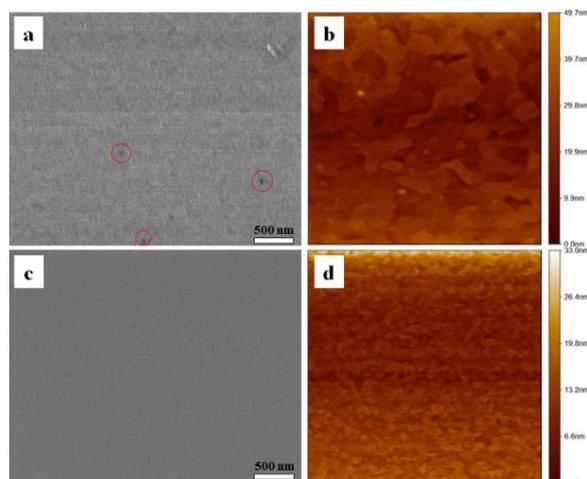
**Fig. 2** Top-view SEM images of (a) bare and (c) passivated SnO<sub>2</sub> films; AFM images of the (b) bare and (d) passivated SnO<sub>2</sub> films.
