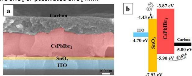
**Fig. 3** (a) Cross-section SEM image and (b) energy diagram of the components of the all-inorganic CsPbIBr<sub>2</sub> PSCs.
