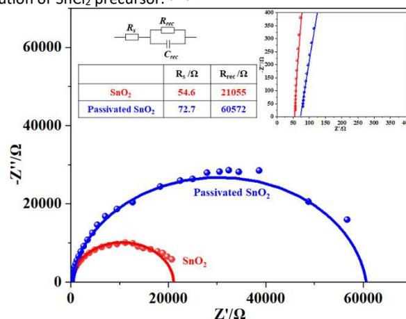
**Fig. 5** Nyquist plots of PSCs based on bare or passivated SnO<sub>2</sub> in dark condition at a voltage of  $V_{oc}$ . Inset: the equivalent circuit, the enlarged high-frequency region, and table of simulated results.
