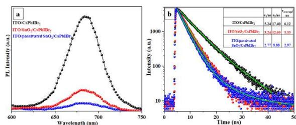
**Fig. 6** (a) Steady-state photoluminescence (PL) spectra and (b) normalized transient PL decay profiles for CsPbI<sub>2</sub>Br<sub>2</sub>, bare SnO<sub>2</sub>/CsPbI<sub>2</sub>Br<sub>2</sub>, and passivated SnO<sub>2</sub>/CsPbI<sub>2</sub>Br<sub>2</sub>.
