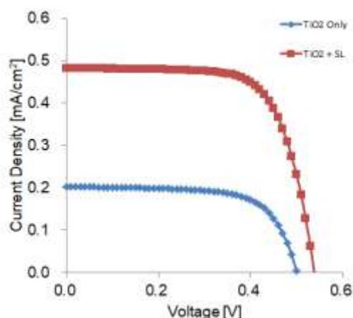
**Figure 2.** I-V Characteristic of DSSCs
