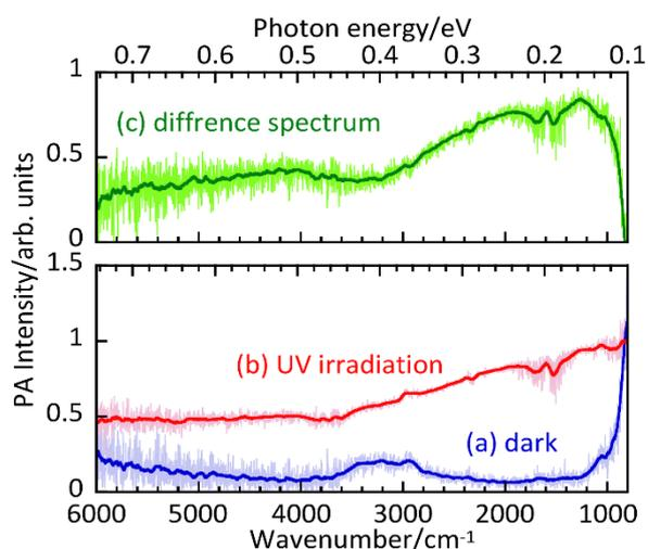
**Fig. 1** FTIR-PAS spectra of anatase TiO<sub>2</sub> (AMT-600) with adsorbed ethanol under nitrogen (a) before and (b) after UV irradiation and (c) difference spectrum between (a) and (b). Blue, red and green lines are smoothed spectra by 33 point moving average of original data (pale blue, pink and yellow green lines).
