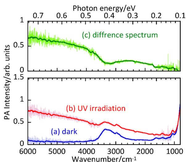
**Fig. 3** FTIR-PAS spectra of rutile  $\text{TiO}_2$  (MT-150A) with adsorbed ethanol under nitrogen (a) before and (b) after UV irradiation and (c) difference spectrum between (a) and (b). Blue, red and green lines are smoothed spectra by 33 point moving average of original data (pale blue, pink and yellow green lines).
