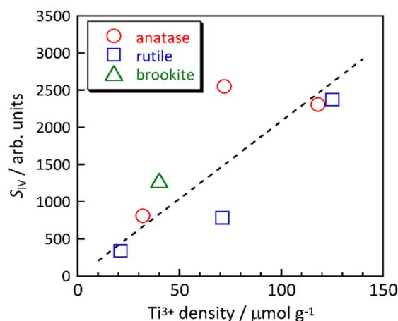
**Fig. 5** Relation between  $S_{IV}$  and  $Ti^{3+}$  density.
