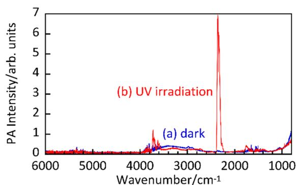
**Fig. 2** FTIR-PAS spectra of anatase TiO<sub>2</sub> (AMT-600) with adsorbed ethanol under oxygen (a) before and (b) after UV irradiation.
