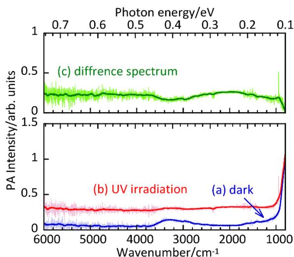
**Fig. 4** FTIR-PAS spectra of brookite TiO<sub>2</sub> with adsorbed ethanol under nitrogen (a) before and (b) after UV irradiation and (c) difference spectrum between (a) and (b). Blue, red and green lines are smoothed spectra by 33 point moving average of original data (pale blue, pink and yellow green lines).
