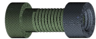
(a) FEM model M12 bolt and nut
