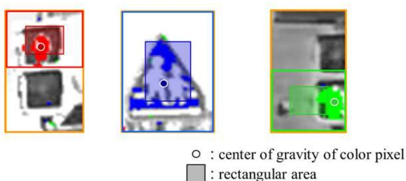
FIGURE 4. The center of gravity of color pixels and a rectangular area
