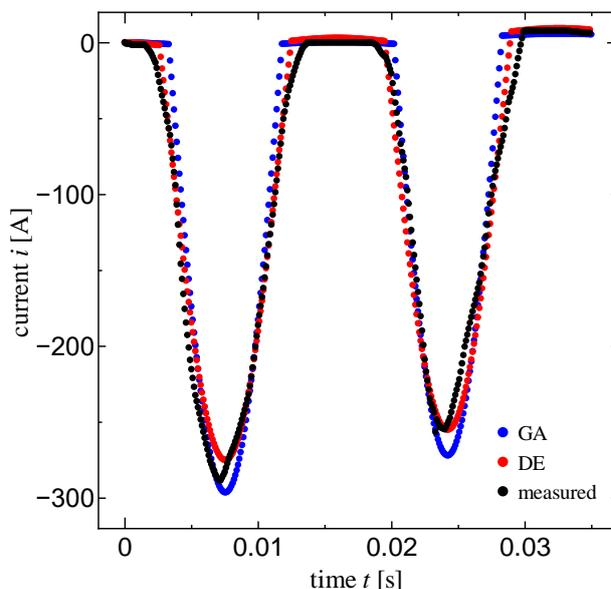
**Figure 3.** Waveform of inrush current for measured and estimated values by GA and DE.
