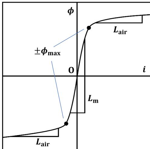
**Figure 2.** Simplified hysteresis of iron core,  $i$ - $\phi$ .
