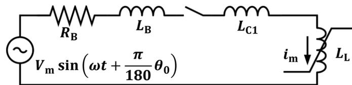
**Figure 1.** Equivalent circuit for single-phase superconducting transformer.
