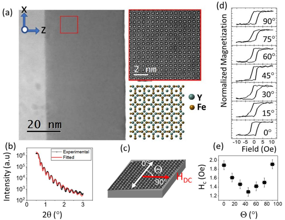
Figure 2. (a) Aberration corrected (AC)- Scanning Transmission Electron Microscopy (STEM) showing the cubic lattice of the 45 nm YIG (001) thin film. (b) X-ray reflectivity measurements of YIG (001)/GGG (001). (c) Schematic showing the in-plane angle ( $\Theta$ ) between the [100] and applied magnetic field. (d) M-H loop and (e) coercive field as a function of  $\Theta$ .
