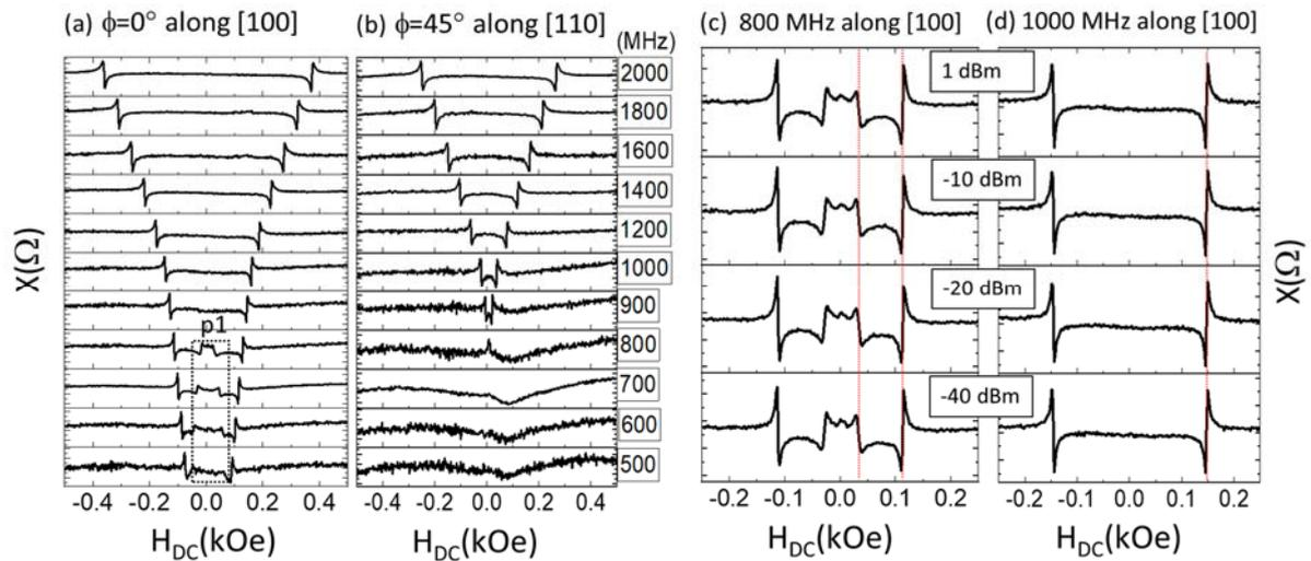
Figure 4. Impedance spectra of the copper strip coil for (a)  $\phi=0^\circ$  along [100] and (b)  $\phi=45^\circ$  along [110]. Power dependent magneto-impedance spectra of the copper strip coil for along YIG [100] direction at (c) 800 MHz and (d) 1000 MHz excitation frequencies.
