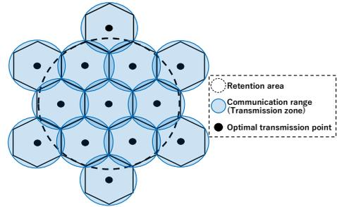
Fig. 2. Regular hexagon type optimal transmission point.
