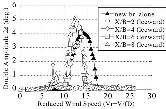
Fig. 9. Torsional response of leeward new bridge
