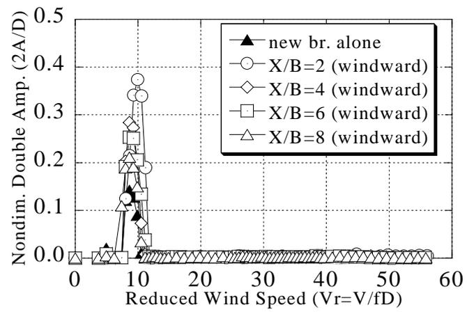
Fig. 3. Heaving response of windward new bridge
