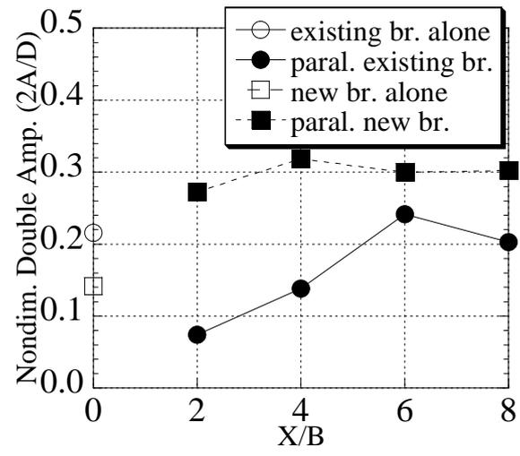
Fig. 7. Maximum heaving response amplitude of leeward bridge
