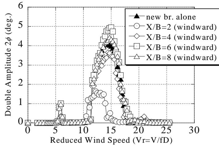
Fig. 8. Torsional response of windward new bridge
