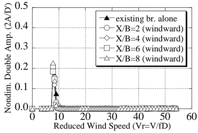
Fig. 2. Heaving response of windward existing bridge
