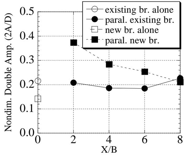
Fig. 4. Maximum heaving response amplitude of windward bridge
