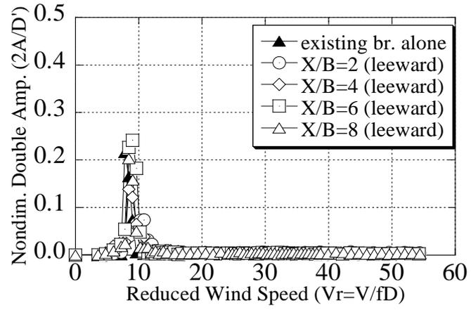
Fig. 5. Heaving response of leeward existing bridge
