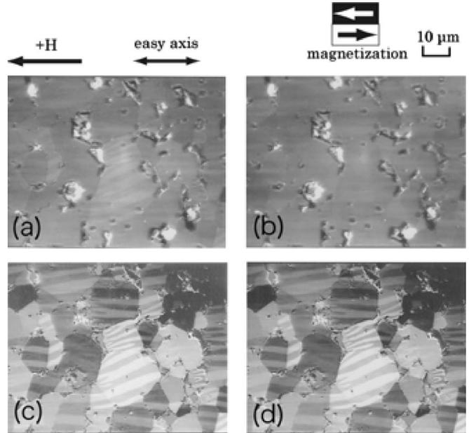
FIG. 4. Domain images by a different image processing technique with a liquid crystal element: (a) live image, (b) reference image, (c) subtracted image, and (d) integrated image.
