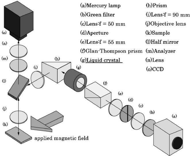
FIG. 2. A schematic diagram of the Kerr-effect microscope with liquid crystal element.
