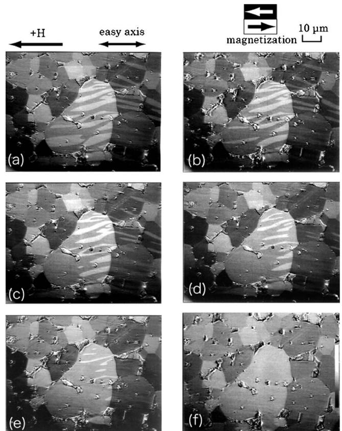
FIG. 5. Magnetization process of Nd-Fe-B sintered magnet: (a)  $H=0$  kOe, (b)  $H=0.3$  kOe, (c)  $H=0.7$  kOe, (d)  $H=1.3$  kOe, (e)  $H=2.0$  kOe, and (f)  $H=4.4$  kOe.
