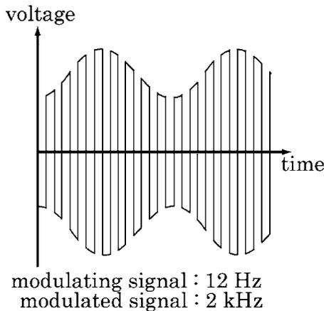
FIG. 3. Wave form of driving voltage for liquid crystal element.
