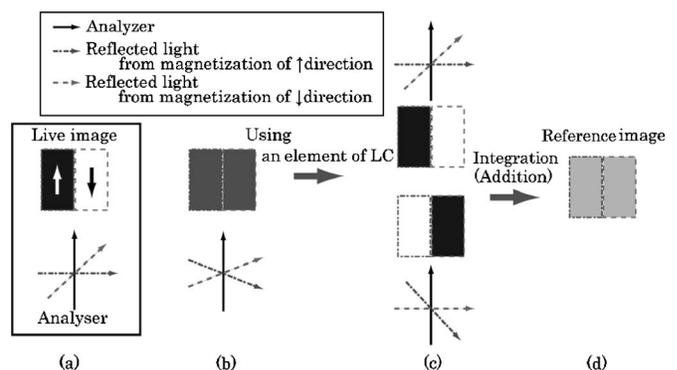
FIG. 1. Principle of reference image acquisition: (a) live image, (b) initial state, (c) modulated image, and (d) reference image.
