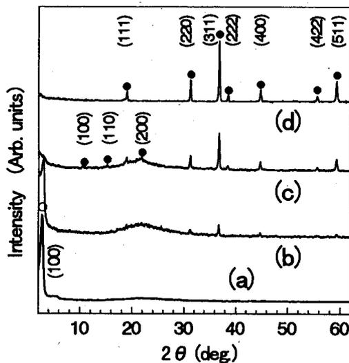
FIG. 1. X-ray diffraction patterns with  $CuK\alpha$  radiation of the molecular sieve (a), the  $Co_3O_4$  diluted systems from the 0.01 mol/l solution (b) and from the 0.1 mol/l solution (c), and the  $Co_3O_4$  powders (d). ●:  $Co_3O_4$  and ○: MCM-41 molecular sieve.
