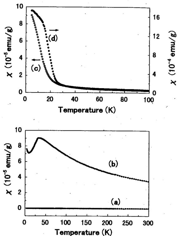
FIG. 2. Temperature dependent dc magnetic susceptibilities in  $H = 1000$  G of the molecular sieve (a) and the  $Co_3O_4$  powders (b) in the lower panel, and those of the  $Co_3O_4$  diluted systems from the 0.01 mol/l solution (c) and the 0.1 mol/l solution (d) in the upper panel.
