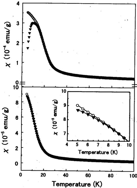
FIG. 3. Temperature dependencies of the field cooled (○) and zero field cooled (▼) susceptibility in  $H=1000$  G of the  $\text{Co}_3\text{O}_4$  diluted systems from the 0.01 mol/l solution (lower panel) and from the 0.1 mol/l solution (upper panel).
