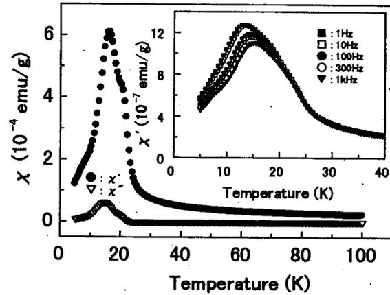
FIG. 5. Temperature dependence of ac susceptibility,  $\chi'$  and  $\chi''$ , in  $H=2$  G and at  $f=100$  Hz of the  $\text{Co}_3\text{O}_4$  diluted system from the 0.1 mol/l solution. Inset: Frequency dependence of the real part of ac susceptibility  $\chi'$  from  $f=1$  to 1000 Hz in  $H=230$  G of the  $\text{Co}_3\text{O}_4$  diluted system from the 0.1 mol/l solution.
