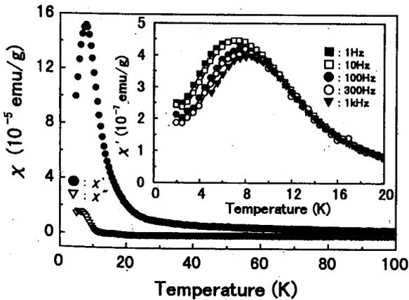
FIG. 4. Temperature dependence of ac susceptibility,  $\chi'$  and  $\chi''$ , in  $H=2$  G and at  $f=100$  Hz of the  $\text{Co}_3\text{O}_4$  diluted system from the 0.01 mol/l solution. Inset: Frequency dependence of the real part of ac susceptibility  $\chi'$  from  $f=1$  to 1000 Hz in  $H=230$  G of the  $\text{Co}_3\text{O}_4$  diluted system from the 0.01 mol/l solution.
