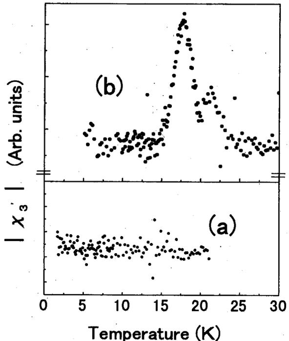
FIG. 6. Temperature dependence of nonlinear susceptibility  $\chi_3'$  ( $3\omega$  signal) at  $f=0.1$  Hz with  $h_0=2$  G of the diluted systems from the 0.01 mol/l solution in 1.7–20 K (a) and from the 0.1 mol/l solution in 5–30 K (b).
